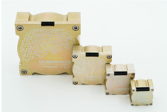
Figure 2.3: CubeWheel hardware in four different sizes. The three wheels on the right side are the CW0162, CW0057 and the CW0017, seen from right to left. [32]
