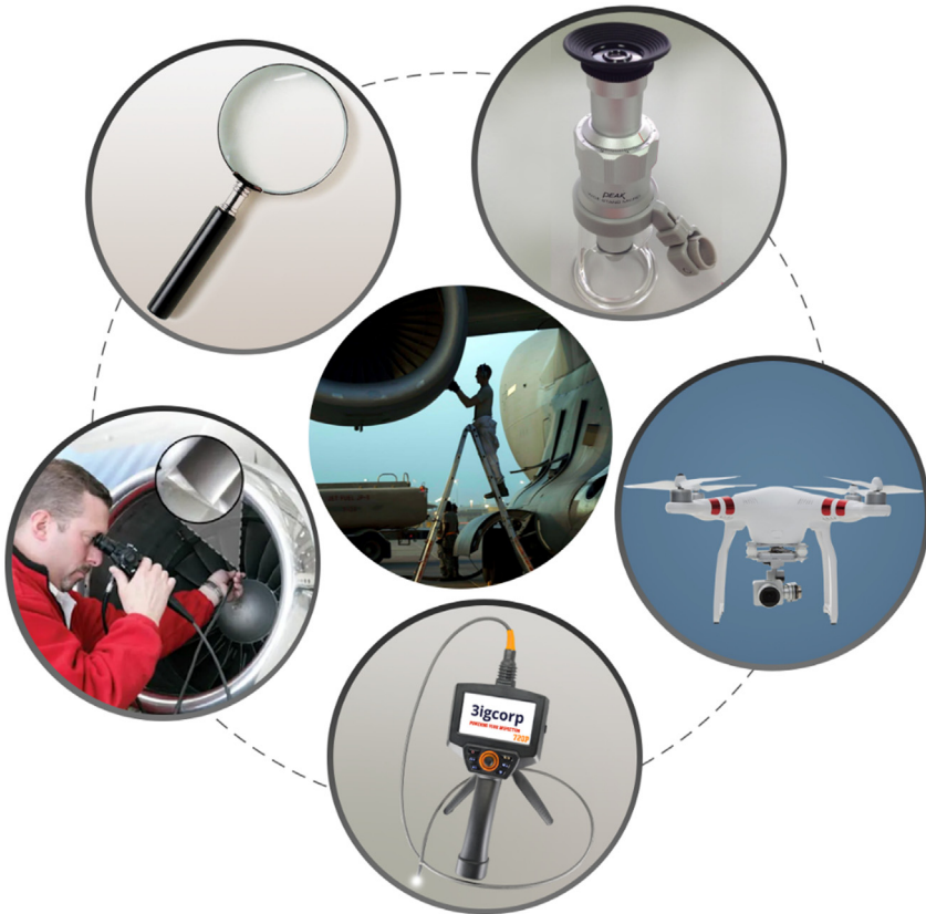
Figure 2.1 Examples of direct (in the center) and assisted visual inspection.
