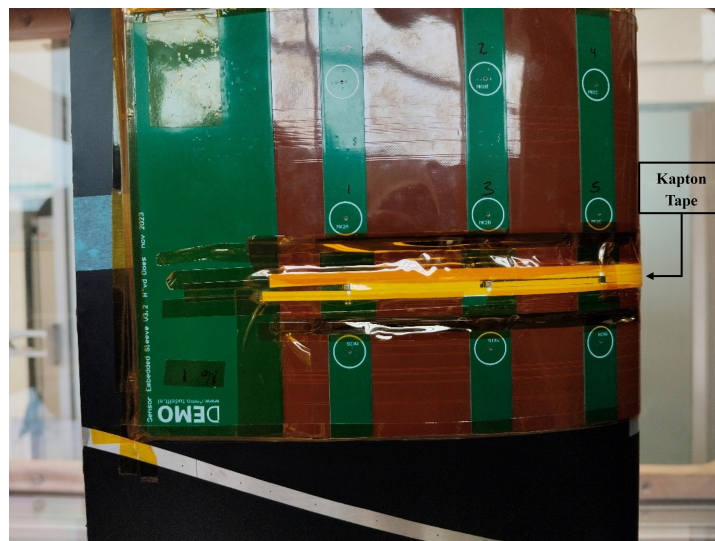
Figure 4.2: The placement of the Kapton tape on the device as viewed from the pressure side of the airfoil model.
