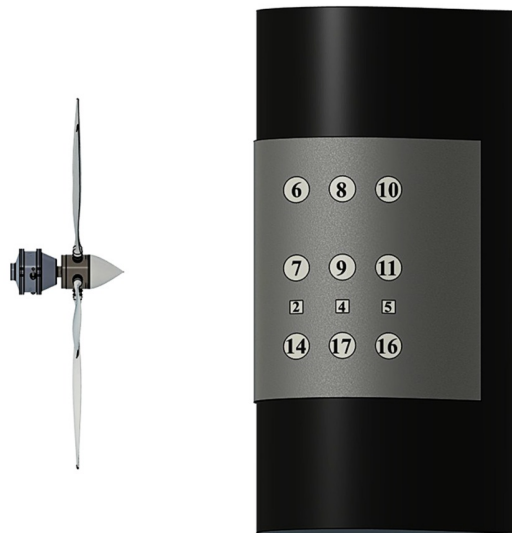
Figure 2.10: Illustration of the device layout when wrapped around the LE of the airfoil model (suction side view). The illustration is not to scale; sensor dimensions and coordinates are exaggerated for clarity. However, the relative ordering and arrangement of the microphones and pressure sensors accurately reflect the physical configuration. Circles represent the microphones and squares represent the pressure sensors, with their respective channel numbers annotated. The propeller shown is for illustrative purposes only and does not represent the geometry or specifications of the TUD XPROP-S.
