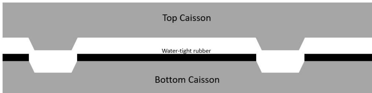
Figure I.19: Side view of bottom and top caisson connection.
