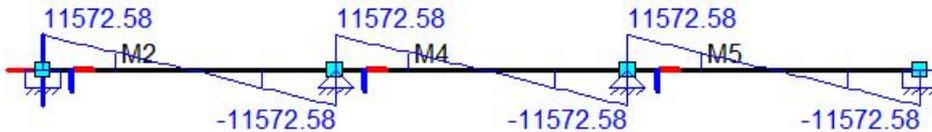
Figure 7.44: Shear force diagram of the water-retaining wall. MatrixFrame output.
