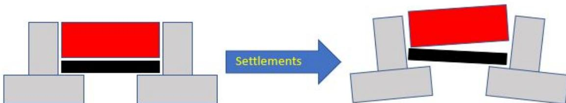
Figure H.1: Settlements affection to closing operation for the Eastern Scheldt barrier.
