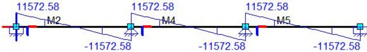
Figure L.84: Shear force diagram from MatrixFrame
