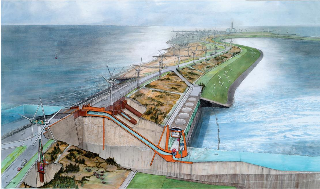
Figure A.6: Dike section of the Valmeer with the pumping system (Illustration by the Das brothers). Source: <https://www.deingenieur.nl/artikel/lievence-de-man-van-het-opslagbekken>
