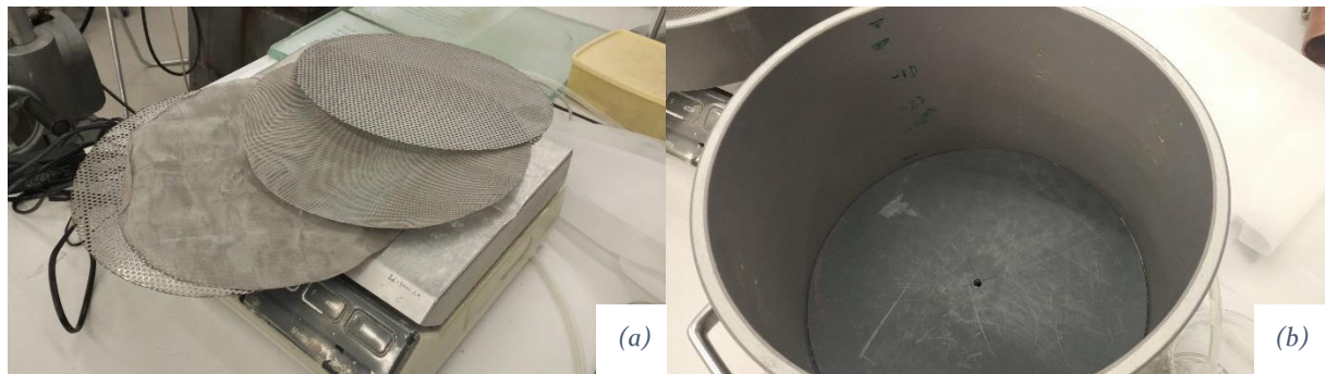
Figure 14 Filtration layer. (a) Four layers of mesh to prevent the outflow of particles. (b) Outflow opening for extracting pore water from the bottom. A 10 mm plastic grid is placed on top of the bottom before placing the layers of mesh.
