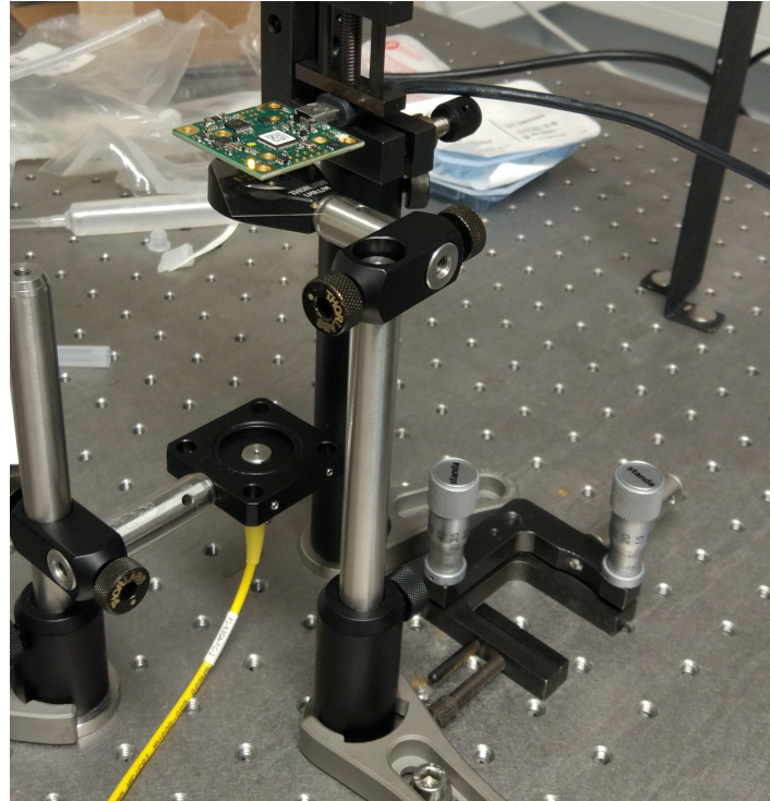
Figure 3-2: The initial configuration of the DHM setup for imaging stationary samples. In this image the object consists of SH eggs between two microscopic glass slides.
