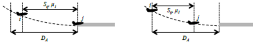
Figure 4.2: Closing case, with a slower leader aircraft j and faster follower i (left) and Opening case, with a faster leader j and slower follower i (right). [22]
