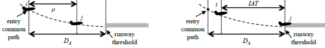
Figure 4.1: Time separation \mu imposed throughout common approach path (left) and Inter-Arrival Time (right). [22]
