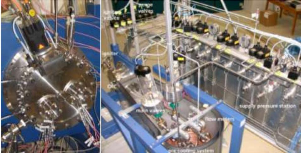
Figure 3.1: Test facility for HF-instabilities research, supply system (right) and CRC (left)
