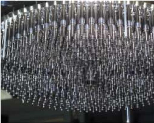
Figure 8.2: Multi-element injector head of Vulcain2 [42]
