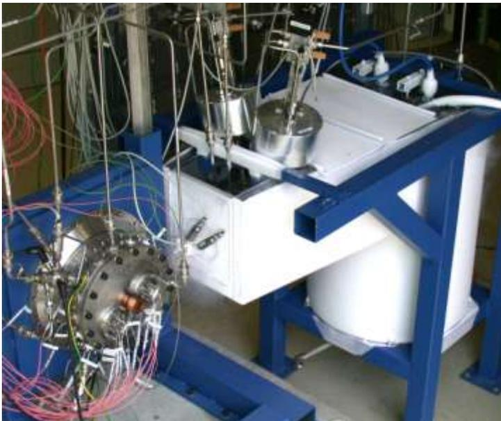
Figure 3.2: Test facility for HF-instabilities research after cool down
