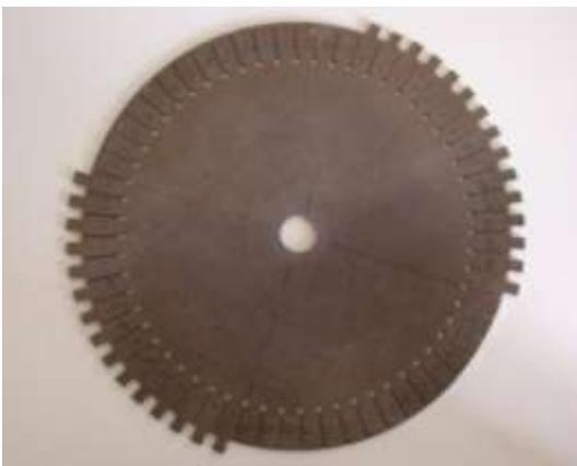
Figure 8.1: Siren wheel for 90 degree excitation
