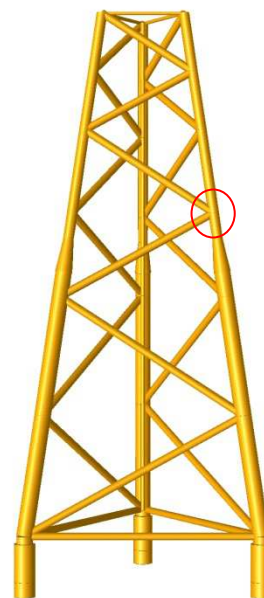
Figure 6.21: 3-Leg jacket with K-braces
