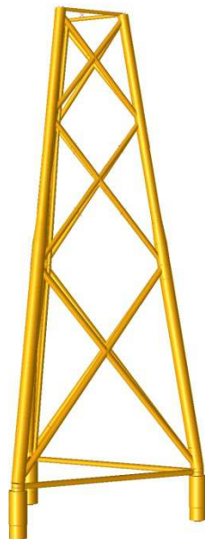
Figure 6.20: 3-Leg jacket with X-braces
