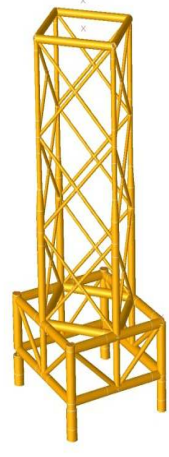
Figure 4.4: 4-leg straight jacket
