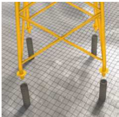
Figure 5.8: Stabbing of legs in piles
