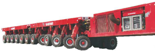
Figure 8.1: Self Propelled Modular Transporter (SPMT)
