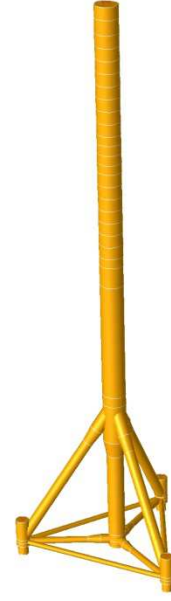
Figure 6.8: Tripod concept large base width
