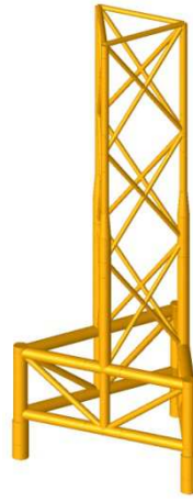
Figure 4.3: 3-leg straight jacket
