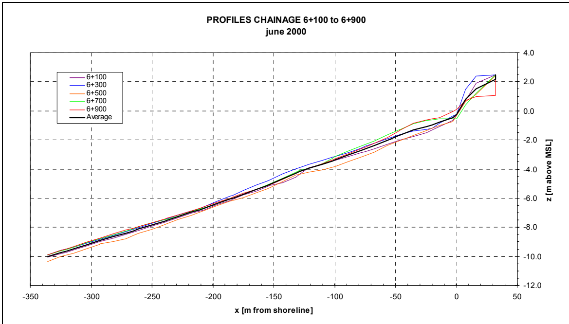
Figure E-5: Individual profiles and averaged profile at June 2000 for chainage 6+100 to 6+900.
