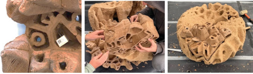
Fig. 4.4 Integration of sensors and batteries (white boxes) in component (left), componential logic (middle), and assembled prototype
