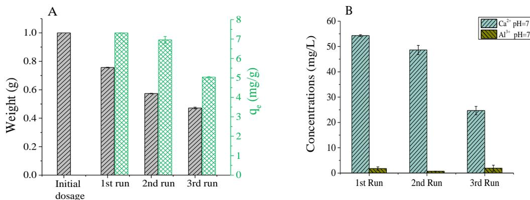
Figure 6. Mass balance,  $q_e$  (A) (Granule dose=1 g/L; F<sup>-</sup>=10mg/L; pH=7; T=20±2°C; Time=30+1 h) and cations dissolution (B) of extrusion granule (95% LDHs) after 3 runs.
