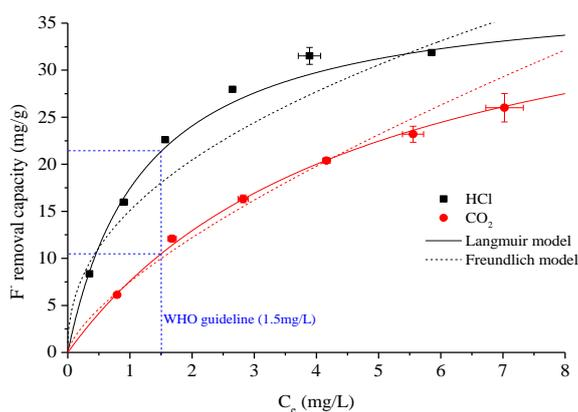
**Figure S2.** Isotherm of F<sup>-</sup> uptake by Ca-Al-CO<sub>3</sub> LDHs under HCl and CO<sub>2</sub> pH adjustment conditions.
