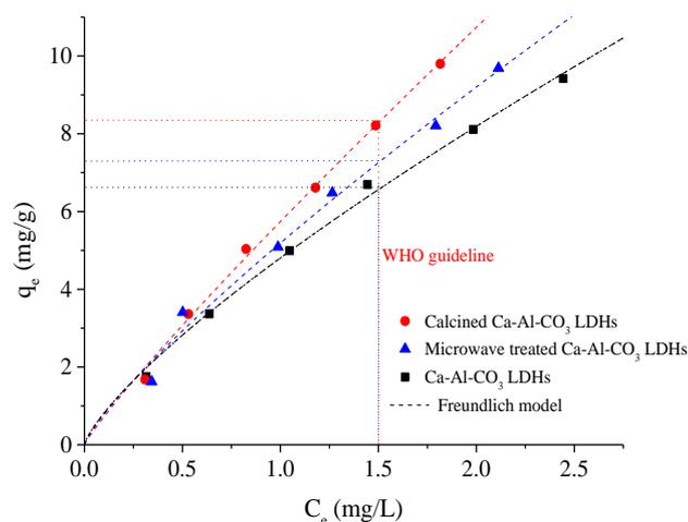
**Fig. 2.**  $\text{F}^-$  adsorption isotherm on Ca-Al- $\text{CO}_3$  LDH and its modified products, with loadings at WHO guideline of 1.5 mg/L value indicated as dashed lines.
