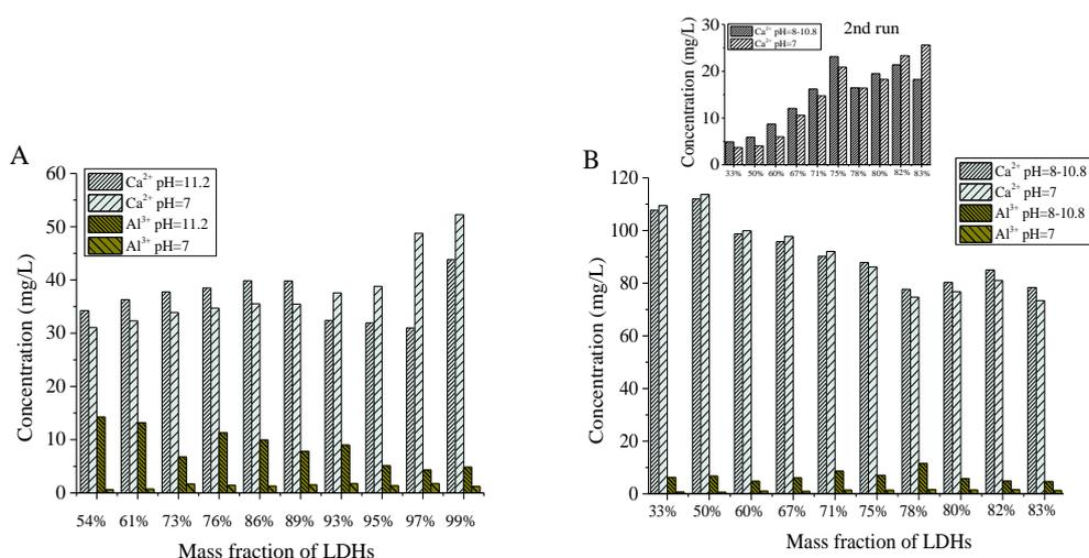
Figure S2.  $\text{Ca}^{2+}$  and  $\text{Al}^{3+}$  leaching from LDHs extrusion granules (A) dropping beads (B) at varying LDH mass fractions and two different pHs. (granular LDHs dosage=1 g/L; 100mL water; temperature= $22^\circ\text{C}$ ; soaked for 30h)
