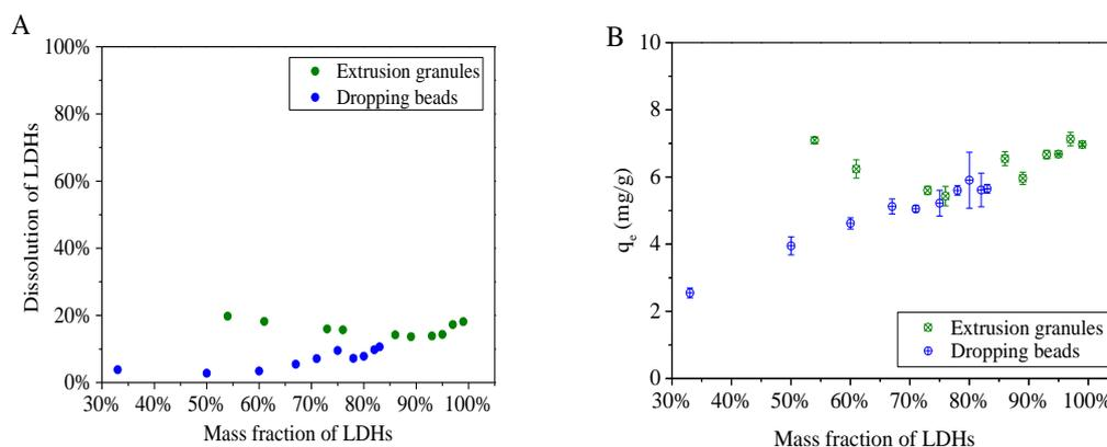
Figure 4. Dissolution (A) and F<sup>-</sup> removal capacity (B) (Granules dose=1 g/L; initial F<sup>-</sup> concentration=10 mg/L; pH=7; temperature=22±2°C) of granular Ca-Al-CO<sub>3</sub> LDHs at varying LDHs mass fractions.
