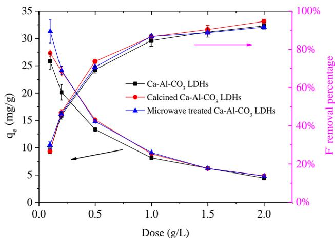
**Fig. S3.** Effect of adsorbent dose on the F<sup>-</sup> removal by Ca-Al-CO<sub>3</sub> LDH and its modified products.
