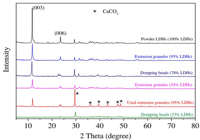
Figure S5. XRD patterns of the powder and granulated Ca-Al-CO<sub>3</sub> LDHs.
