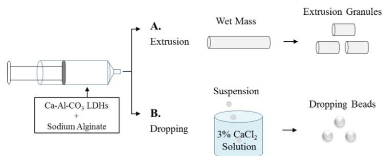
Figure 2. Steps taken to granulate Ca-Al-CO<sub>3</sub> LDHs with sodium alginate by means of extrusion (A) and dropping (B).
