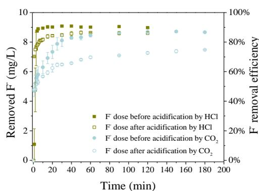
Figure 4. F<sup>-</sup> removal capacity and removal percentage, as a function of time. Initial F<sup>-</sup>=10 mg/L; pH=6; LDHs dose=1 g/L; T=22±1 °C.
