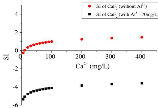
**Figure S5.** The SI values of  $CaF_2$  with and without  $Al^{3+}$ . (pH=6,  $F^-$ =10mg/L,  $T=25^\circ C$ )
