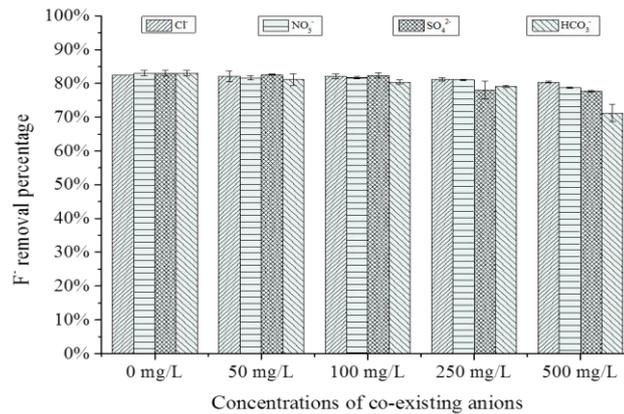
**Fig. 5.** Effect of co-existing anions on the F<sup>-</sup> removal by unmodified Ca-Al-CO<sub>3</sub> LDH. (Initial F<sup>-</sup>=10 mg/L; pH=8; adsorbent dose=1 g/L; T=25±1°C)
