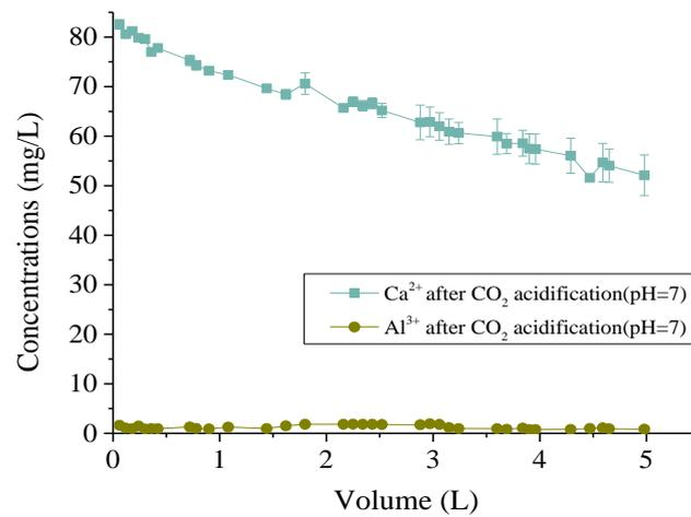
Figure 8. Concentrations of  $\text{Ca}^{2+}$  and  $\text{Al}^{3+}$  from the packed LDH bed effluent after  $\text{CO}_2$  post-acidification. ( $C_0=5\text{mgF}^-/\text{L}$ , influent  $\text{pH}\approx 7$ , Flow= $0.5\text{mL}/\text{min}$ )
