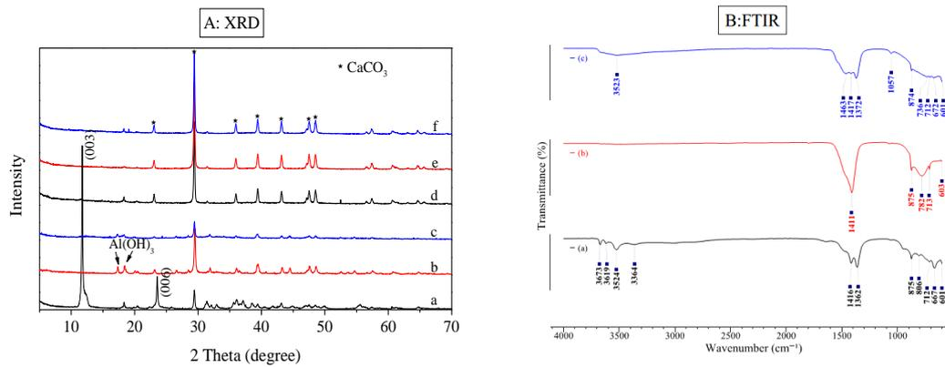
**Fig. 1.** XRD (A) and FTIR(B) spectra of Ca-Al-CO<sub>3</sub> LDHs (a), calcined Ca-Al-CO<sub>3</sub> LDHs (b) and microwave treated Ca-Al-CO<sub>3</sub> LDHs (c), Ca-Al-CO<sub>3</sub> LDHs after adsorption (d), calcined Ca-Al-CO<sub>3</sub> LDHs after adsorption (e) and microwave treated Ca-Al-CO<sub>3</sub> LDHs after adsorption (f); FTIR only measured before adsorption.
