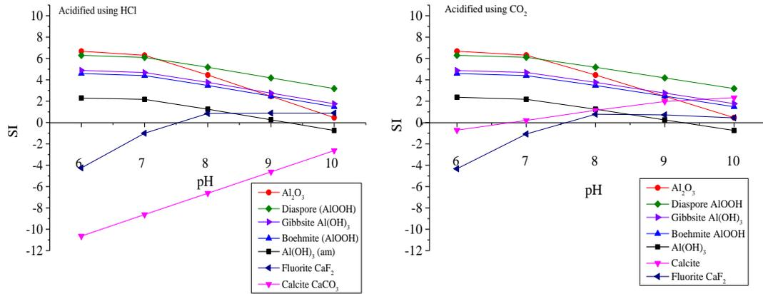
**Figure S6.** Effect of pH on the SI values of Al and Ca species. (T=25°C, pH=6-10, F<sup>-</sup>=10mg/L, molar ratio of F<sup>-</sup>/Al<sup>3+</sup>=0.71).
