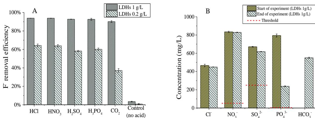
Figure 2. (A)  $\text{F}^-$  removal efficiency at 0.2 and 1 mg/L LDHs dose, and (B) anion concentration of different pH-adjusting acids at start and end of the experiment. Initial  $\text{F}^- = 10 \text{ mg/L}$ , initial  $\text{pH} = 6$ ,  $T = 22 \pm 1^\circ\text{C}$ , LDHs dose = 0.2 or 1 g/L.
