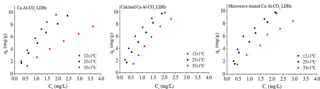
**Fig. 3.** Effect of temperature on the  $F^-$  removal by  $Ca-Al-CO_3$  LDH and its modified products. (Initial  $F^-$ =2,4,6,8,10,12 mg/L; pH=8; adsorbent dose=1 g/L)
