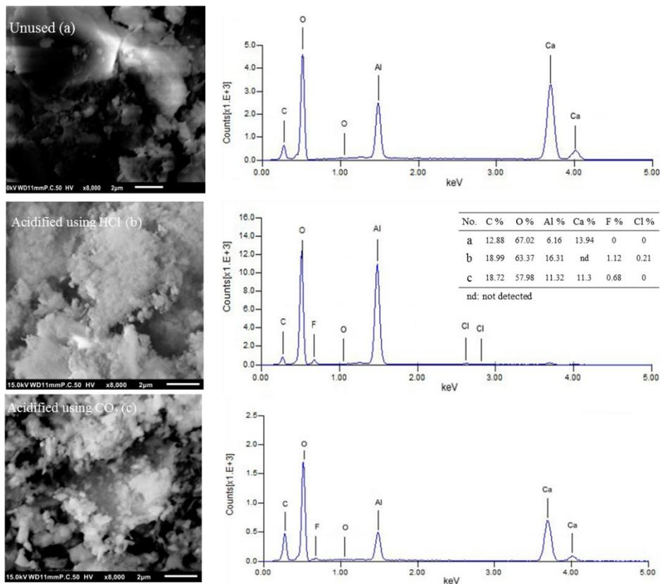
**Figure S7.** SEM images and corresponding EDX spectrum of Ca-Al-CO<sub>3</sub> LDHs before and after experiment (inset: the EDX results (atom%)).
