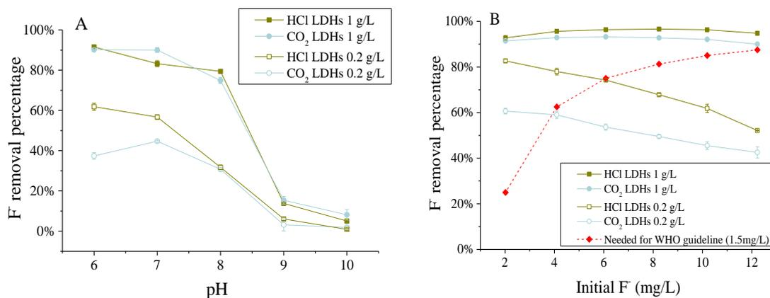
Figure 3. The effect of pH (A) (Initial  $F^-$ =10 mg/L; pH=6, 7, 8, 9, 10; LDHs dose=0.2 g/L;  $T=22\pm 1^\circ C$ ) and initial  $F^-$  (B) (LDHs Initial  $F^-$ =2,4,6,8,10,12 mg/L; pH=6; LDHs dose=0.2 or 1 g/L;  $T=22\pm 1^\circ C$ ) on  $F^-$  removal by Ca-Al- $CO_3$ .
