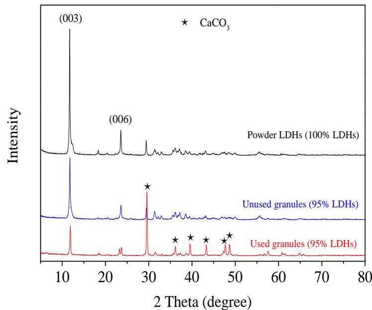
Figure 10. XRD patterns of the powder LDHs and unused/used granules (95% LDHs).
