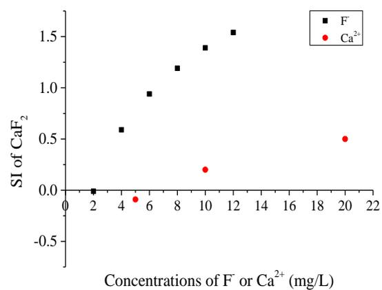
**Fig. S5.** The effect of F<sup>-</sup> and Ca<sup>2+</sup> concentrations on the saturation-index value of CaF<sub>2</sub>.
