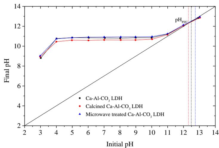
**Fig. S4.** The pH of the point of zero charge (pH<sub>pzc</sub>) of Ca-Al-CO<sub>3</sub> LDHs and its modified products.
