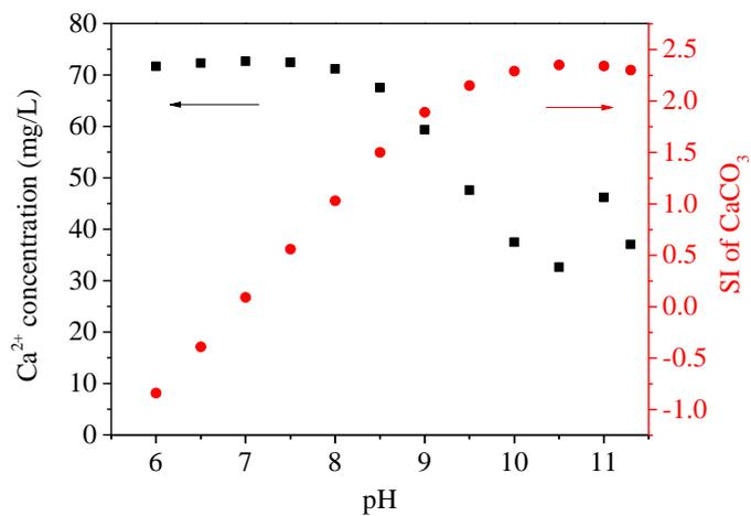
Figure S4. Ca<sup>2+</sup> concentrations and the saturation-index (SI) of CaCO<sub>3</sub> at different pH.
