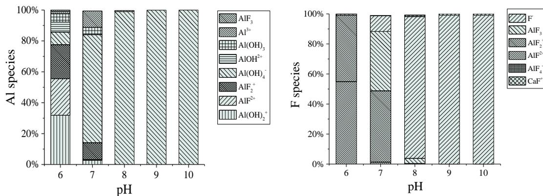
Figure 6. Distribution of Al and F species under different pH conditions simulated by PHREEQC.  $T=25^\circ\text{C}$ ,  $\text{pH}=6\text{-}10$ ,  $\text{F}^-=10\text{ mg/L}$ , the molar ratio of  $\text{F}^-/\text{Al}^{3+}=0.2$ .
