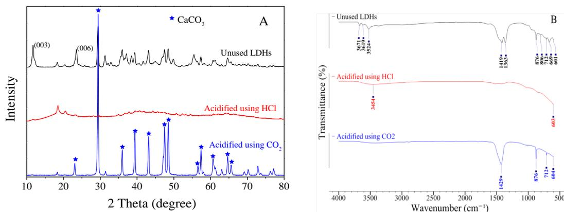
Figure 8. XRD patterns (A) and FTIR spectra (B) of the Ca-Al-CO<sub>3</sub> LDHs before and after experiments.
