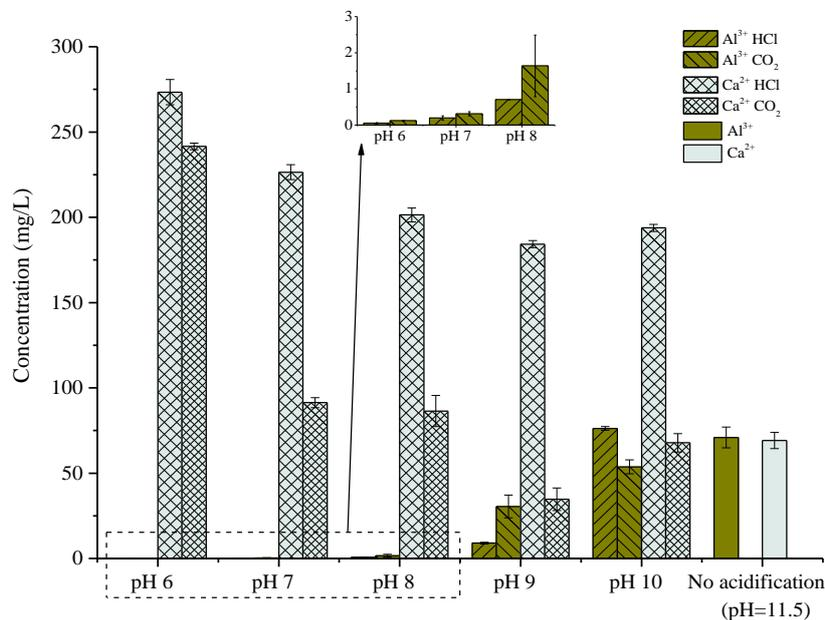
Figure 5. Al<sup>3+</sup> and Ca<sup>2+</sup> leaching from Ca-Al-CO<sub>3</sub> LDHs under different pH conditions; inset: Al<sup>3+</sup> concentrations for pH 6, 7, 8. Initial F<sup>-</sup>=10 mg/L, T=22±1°C, LDHs dose=1 g/L.
