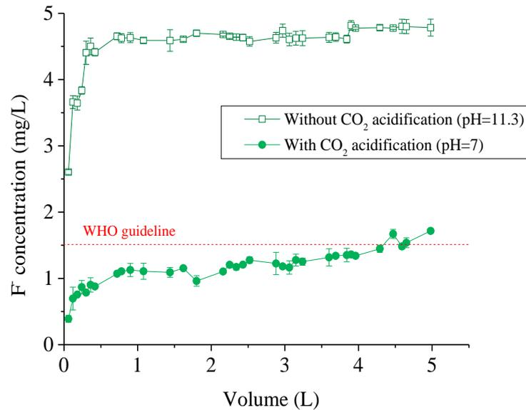
Figure 7. Concentrations of F<sup>-</sup> from the effluent with/without CO<sub>2</sub> acidification and microfiltration. (C<sub>0</sub>=5mgF<sup>-</sup>/L, influent pH≈7, Flow=0.5mL/min)
