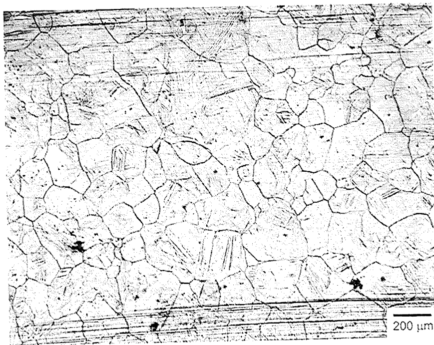
Fig. 5.6: Austenite grain structure (500 x) after annealing at 1473 K.
