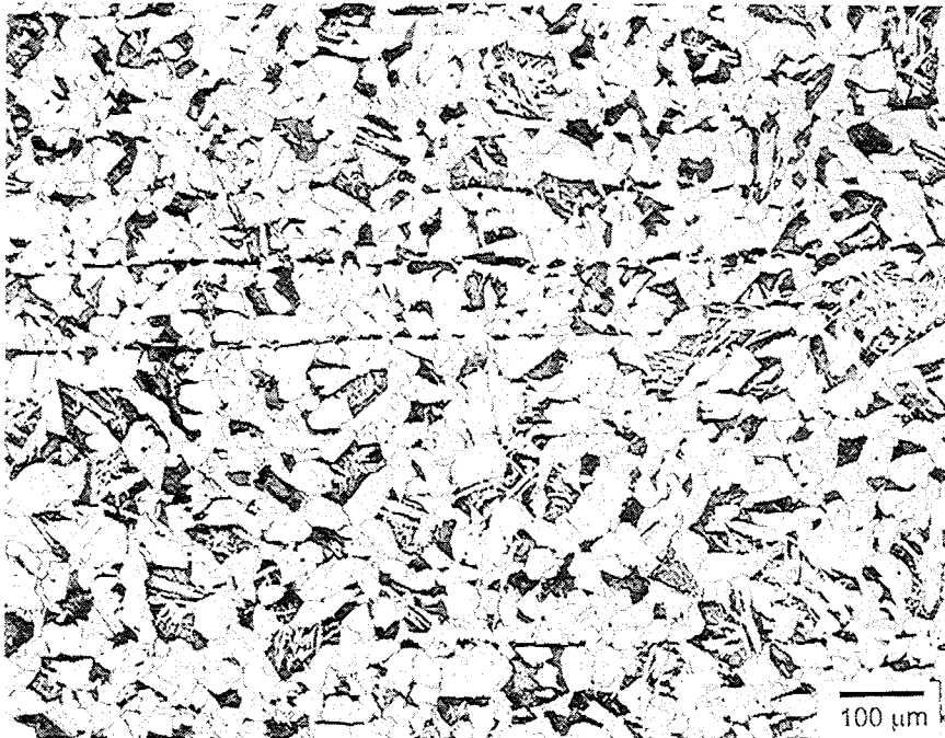
Fig. 5.7: The microstructure (200 x) after annealing at 1273 K and cooling down at 20 K/min, consisting of allotriomorphic ferrite (the white grains) and pearlite (the dark area's).
