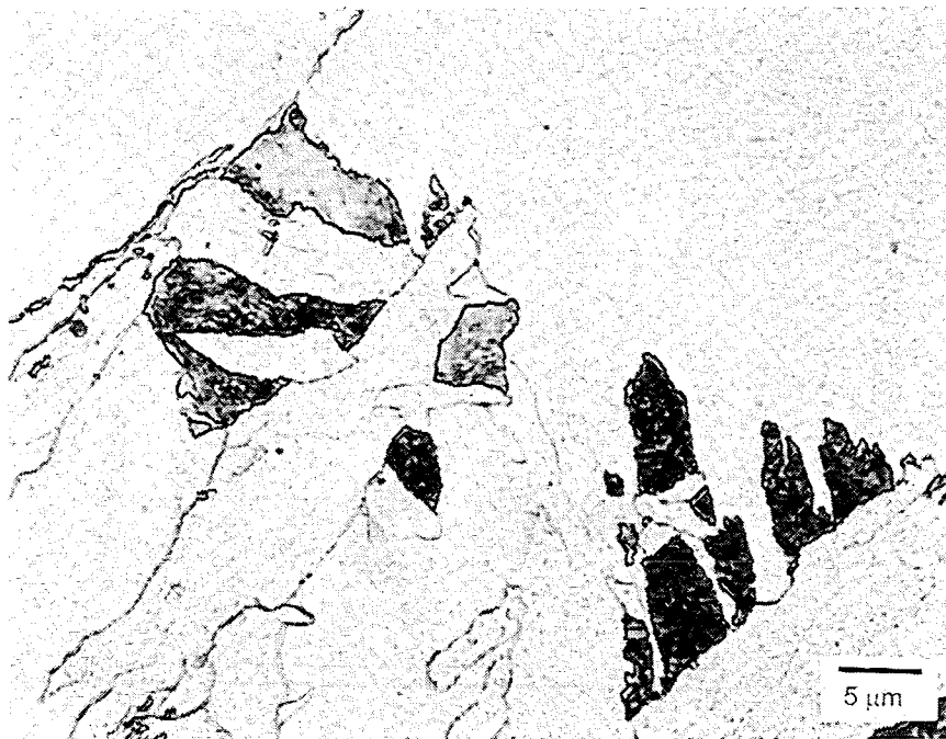
Fig. 5.11: The microstructure (100 x) after annealing at 1523 K and cooling down at 20 K/min consisting of a small layer of allotriomorphic ferrite at the austenite grain boundary, and in the centre of the former austenite grains a mixture of Widmannstätten ferrite, pearlite and bainite.
