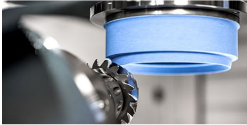
Figure 4.3: Discontinuous generation grinding of pinion using 3M Cubitron II grinding wheel (3M company)
