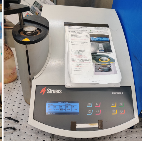
Figure 4.10: The Struers CitoPress-5 machine is used to mount the cut sample into the resin
