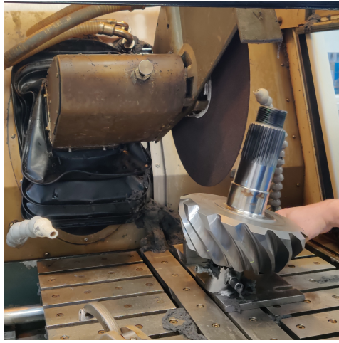
Figure 4.9: the Struers Extom-150 cutting machine uses a feed rate of 0.10 mm/s is used
