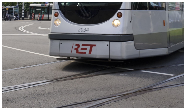
Figure 3.1: RET Alstom Citadis - Protective Shield (based on [25])
