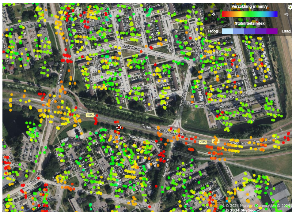
Figure 2.6: InSAR settlement data of the Groeninx van Zoelenlaan [4]
