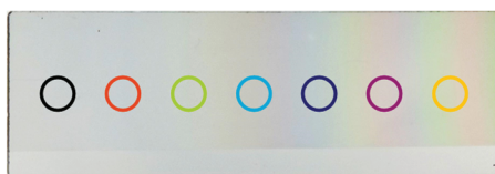
Figure 4.14. 91–428 nm-thick \text{YO}_x\text{H}_y gradient film (see section 3.1.4) sputter-deposited onto f-SiO 2 at a pressure of 0.52 Pa. The black circle corresponds to the thin, porous end of the film and the yellow circle marks the thick, dense end.
