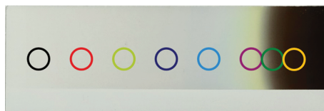
Figure 4.17. 27–119 nm-thick \text{YH}_y – \text{YO}_x\text{H}_y gradient film sputter-deposited onto f- \text{SiO}_2 at a pressure of 0.31 Pa. The transparent parts of the film have fully transformed to \text{YO}_x\text{H}_y upon air exposure, whereas the dark end marked by the yellow circle remains (mostly) \text{YH}_y . The sample positions indicated by the purple and green circles consist of a superposition of both untransformed \text{YH}_y and transformed \text{YO}_x\text{H}_y phases.
