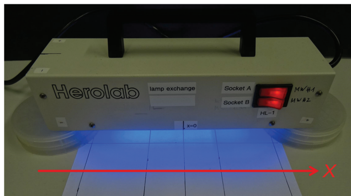
Figure 3.16. Setup used for single-sided MW–MW UV illumination of elongated 76 mm \times 26 mm gradient samples. A single sample is placed along the x -axis at 2.5 cm underneath the lamp, centred around x = 0 with the film facing the lamp.
