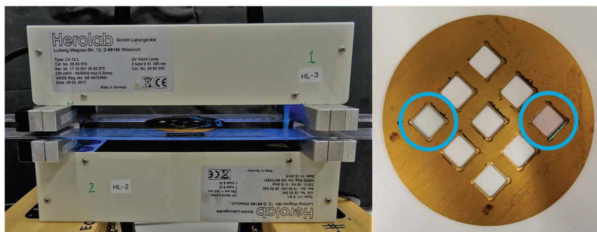
Figure 3.14. Setup used for two-sided (front and back) UV illumination of the 10 mm × 10 mm uniform samples. Up to two samples are inserted at the sample holder positions indicated by the blue circles (right) such that they are at equal distances from the centre of the lamps (coinciding with the centre position on the holder), with the films facing upwards. This way the samples are subjected to roughly equal UV intensities (see Figure 3.17b). The sample holder is positioned between the lamps on two linear scales.
