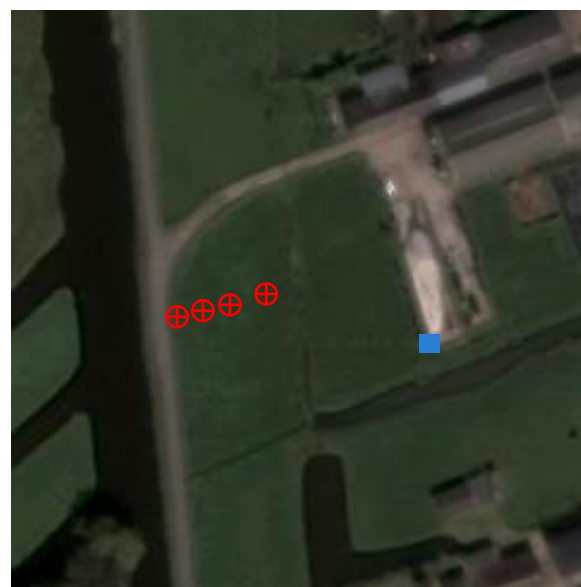
Figure 4.4: Location of the monitoring wells and the rain gauge (blue square) at the Hogedijk.
