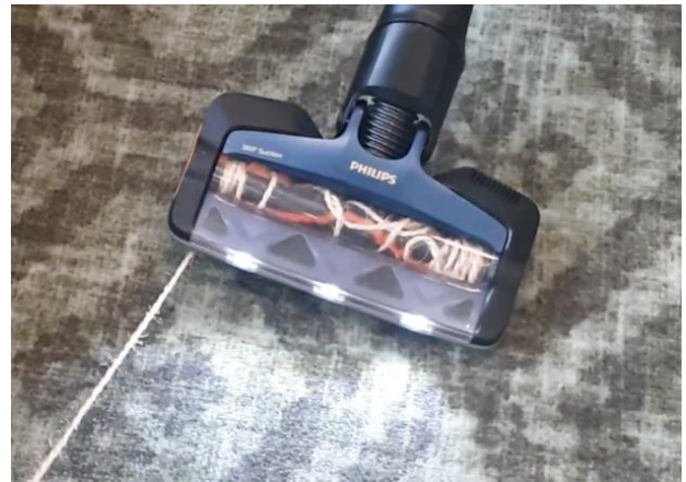
Figure 31: Brush stoppage test, where a cord entanglement causes the brush to stop, thus exerting sudden stress to drivehead.
