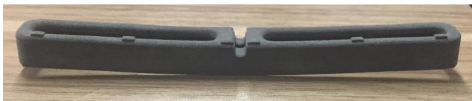
Figure 8: Printed component presenting a deviation from intended dimensions due to warping (Formlabs, n.d.)
