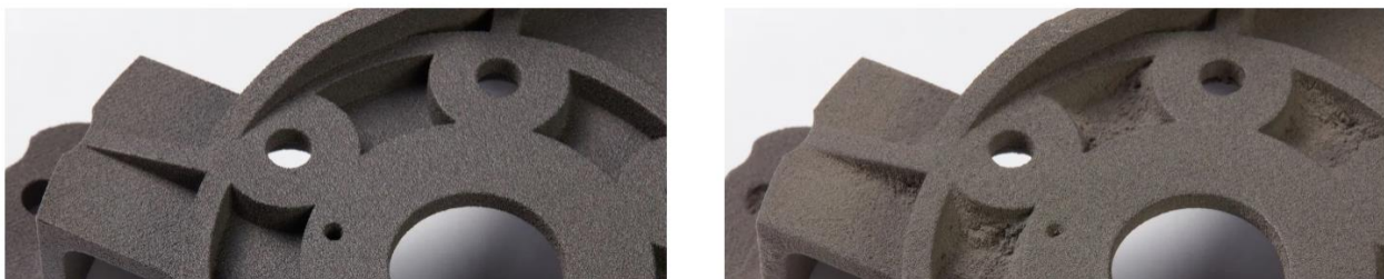
Figure 6: Sand blasted (Left) compared to a component extracted directly from the build chamber, where the Surface Armour can be seen in the cavities (Right). (Image credit: Formlabs)
