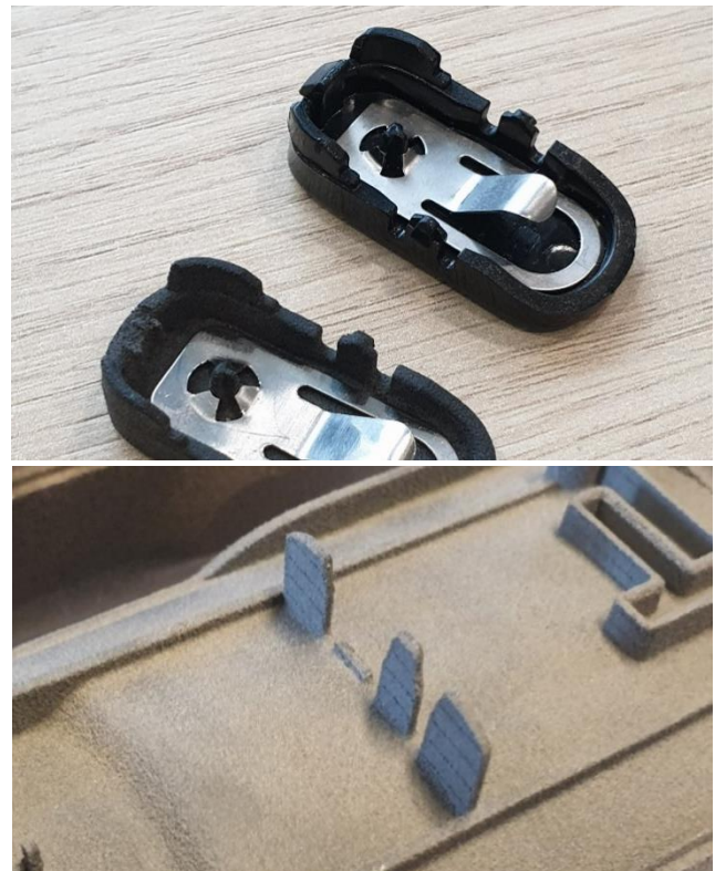
Figure 32: Examples of observed part damage after assembly testing. (Top) The printed components rear hook failed under light load (Bottom) Tube ends present broken thin-walled cable routing feature.
