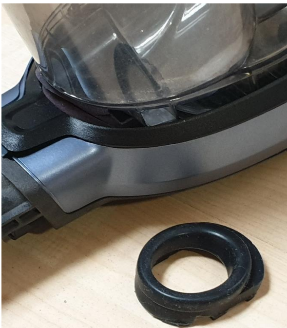
Figure 45: The TPE powder, despite being more flexible than TPU does not accomplish the flexibility requirement of the original motor suspension (Left) and bucket inlet seal (Right).
