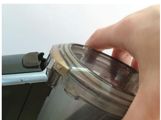
Figure 30: Printed bucket release assembly. Despite its reduced responsiveness it allows for the detachment and lock of the bucket.
