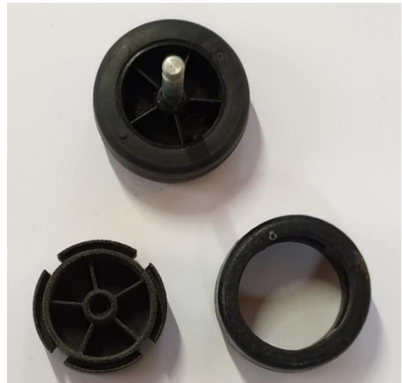
Figure 43: Overview of wheel assembly. Where a core (Left) and the tire (Right) company the multi-material wheel (middle)
