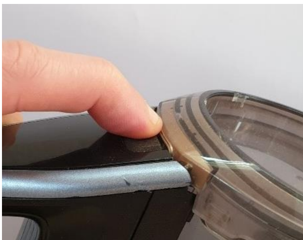
Figure 30: Printed bucket release assembly. Despite its reduced responsiveness it allows for the detachment and lock of the bucket.
