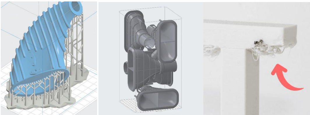
Figure 7: Example of support needed for print in SLA (Left), compared to the building volume and freedom of SLS (Middle). (Right) Example of a FDM failed print due to an unsupported overhanging feature. (Image credit: Left and Middle: Formlabs. Right: 3D Hubs)
