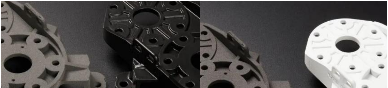
Figure 5: (Left) Vapour smoothed component presenting an IM-like surface finish. (Right) Ceramic coating which enhances part abrasion resistance as well as providing smooth surface (Xometry, n.d.; Formlabs, n.d.) (Image credit: Formlabs)
