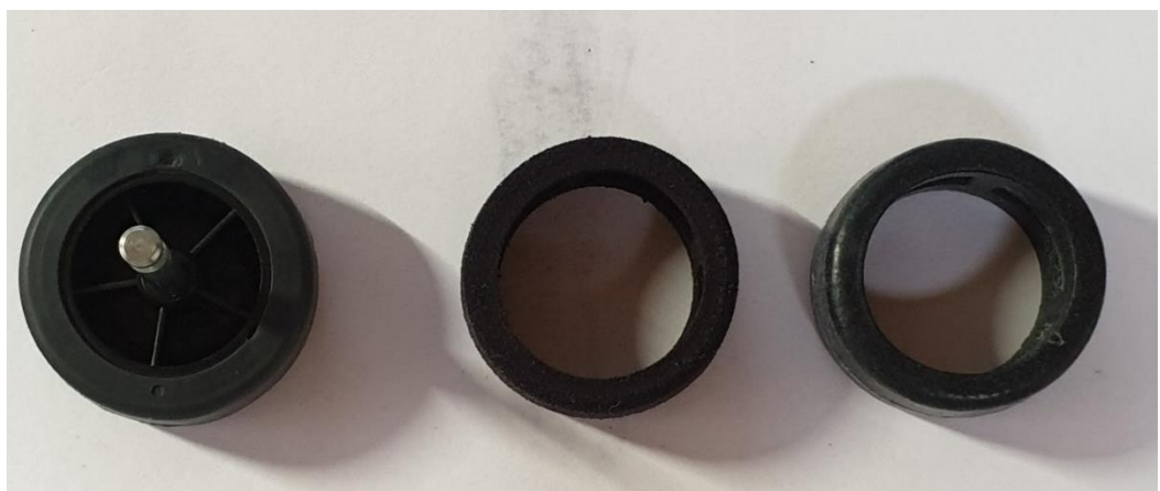
Figure 44: TPE printed wheel rubber (middle) leaves a dark stain when rubbed against a piece of paper, while TPU printed rubber (Right) presents no stain.
