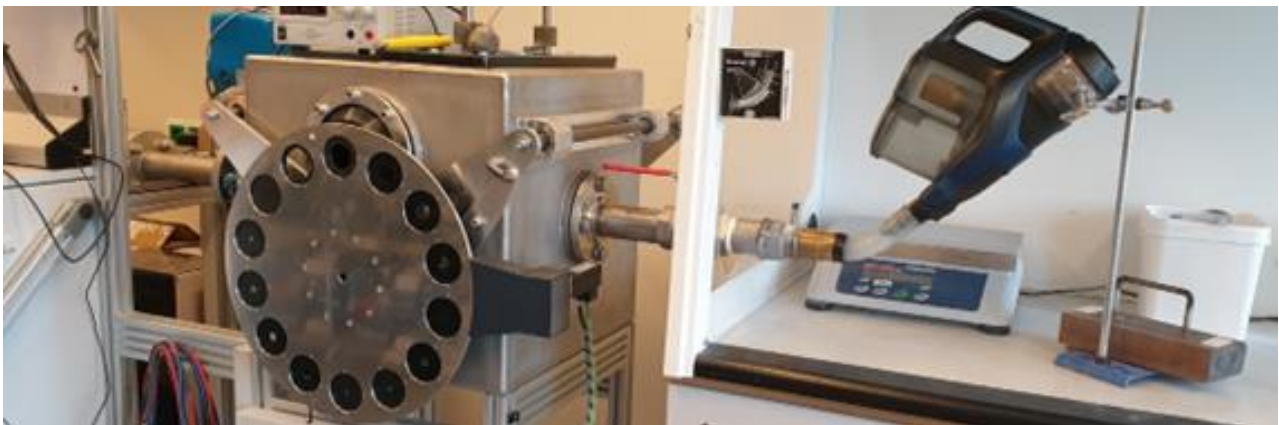
Figure 14: Airflow test setup, where the SPM is connected to the measuring system.
