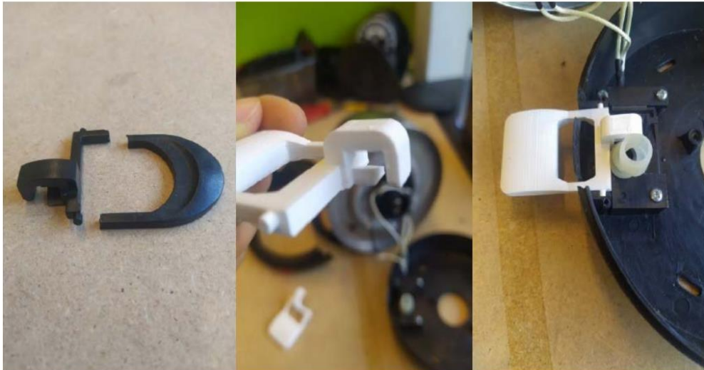
image / figure 1: Example of 3D printed spar parts. (TU Delft SDE department research)
