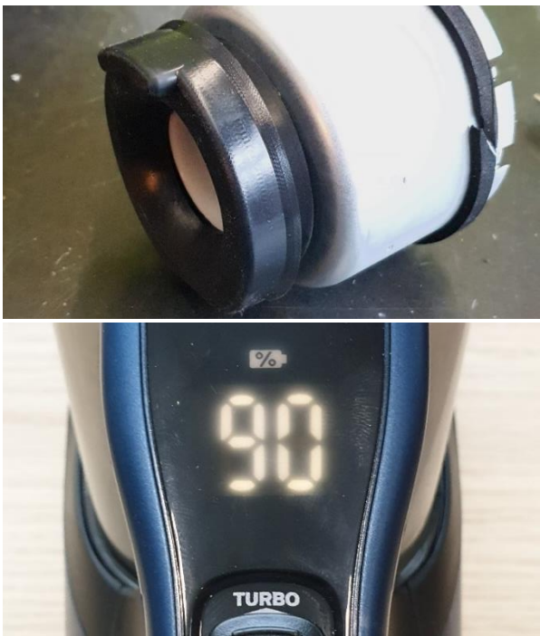
Figure 19: (Top) Motor suspension rubber made from SBR. Its high flexibility allows to mitigate motor vibrations to the rest of the body. (Bottom) Transparent UI window over moulded in the handheld cover.
