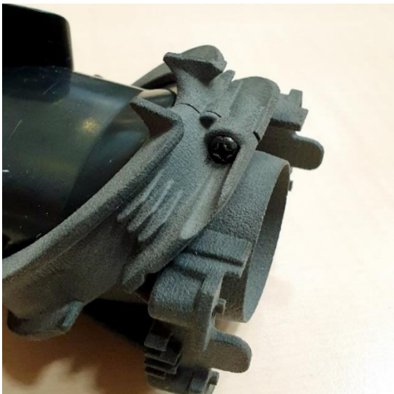
Figure 29: (Left) Printed Nozzle rotation assembly tested with the printed wheel bearings (Right) during simulated vacuuming of company Home Labs.
