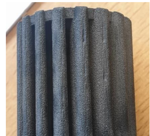
Figure 26 20: Overview of the identified print failures (Top) Resulting cleaning of excess of material in rear wheels cavities. (Middle) Drivehead flat surface warped. (Bottom) Vortex finder presenting poor finish on vertical surface due to bad mix of new and recycle.
