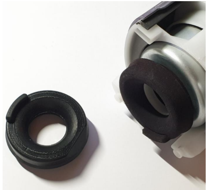
Figure 45: The TPE powder, despite being more flexible than TPU does not accomplish the flexibility requirement of the original motor suspension (Left) and bucket inlet seal (Right).
