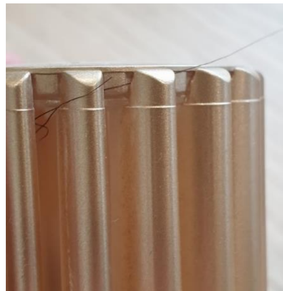
Figure 34: Original vortex finder sample presented particles entangle in its two-part joint section.
