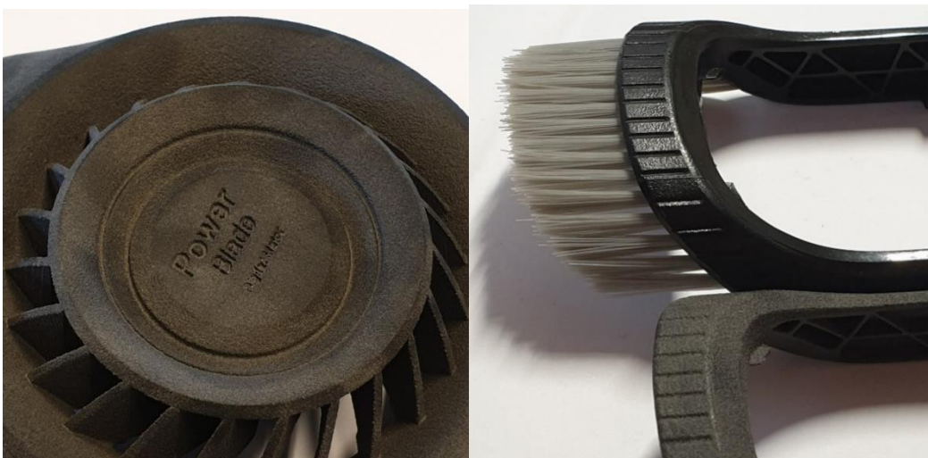
Figure 19: Examples of achieved details. (Top) Motor exhaust grill with proposed embedded text. (Bottom) GF 12 integrated brush with original pattern.
