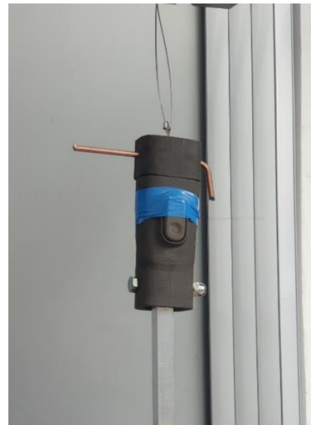
Figure 41:(Left) Obtained results from conducted strain test (Right) Strain setup with designed tube inlet-end connection.
