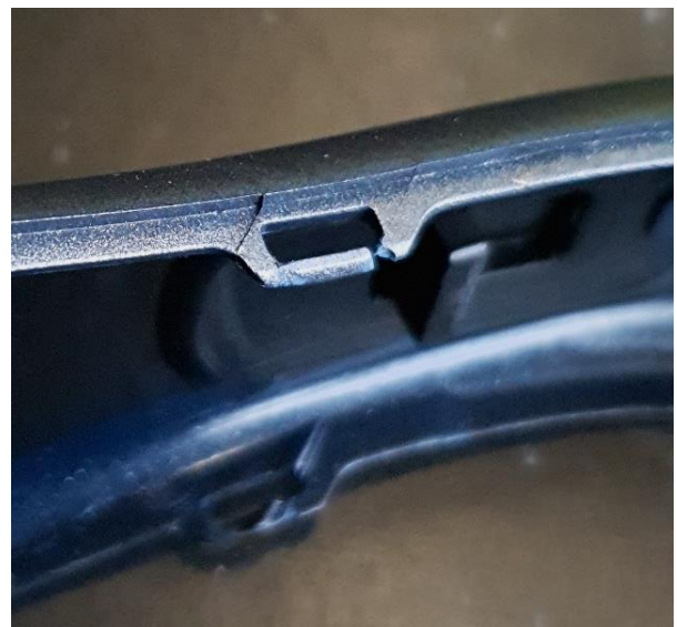
Figure 20: Close up on the damaged snap-fits of the handle cover.
