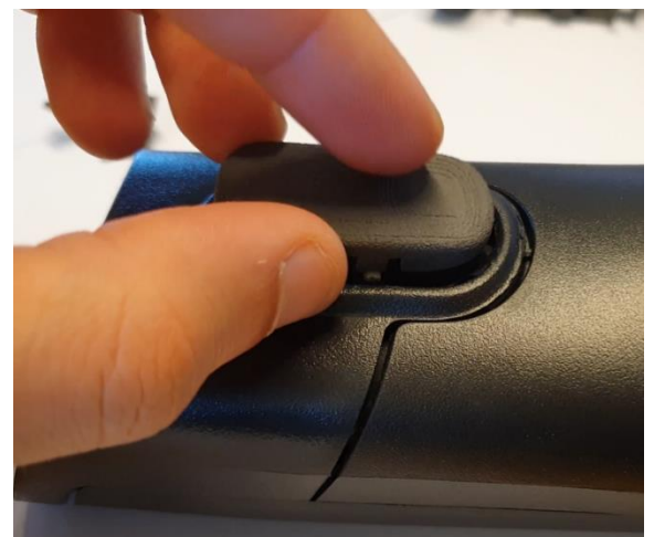
Figure 27: Comparison between original and printed brush (Top). Tube end where the original covers and screws fit as required (Middle). Evaluation of button fit in nozzle end, leading to a successful result.
