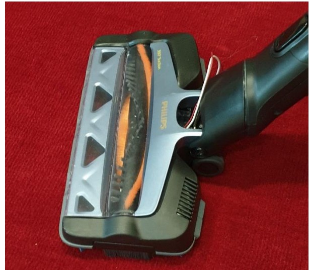
Figure 29: (Left) Printed Nozzle rotation assembly tested with the printed wheel bearings (Right) during simulated vacuuming of company Home Labs.
