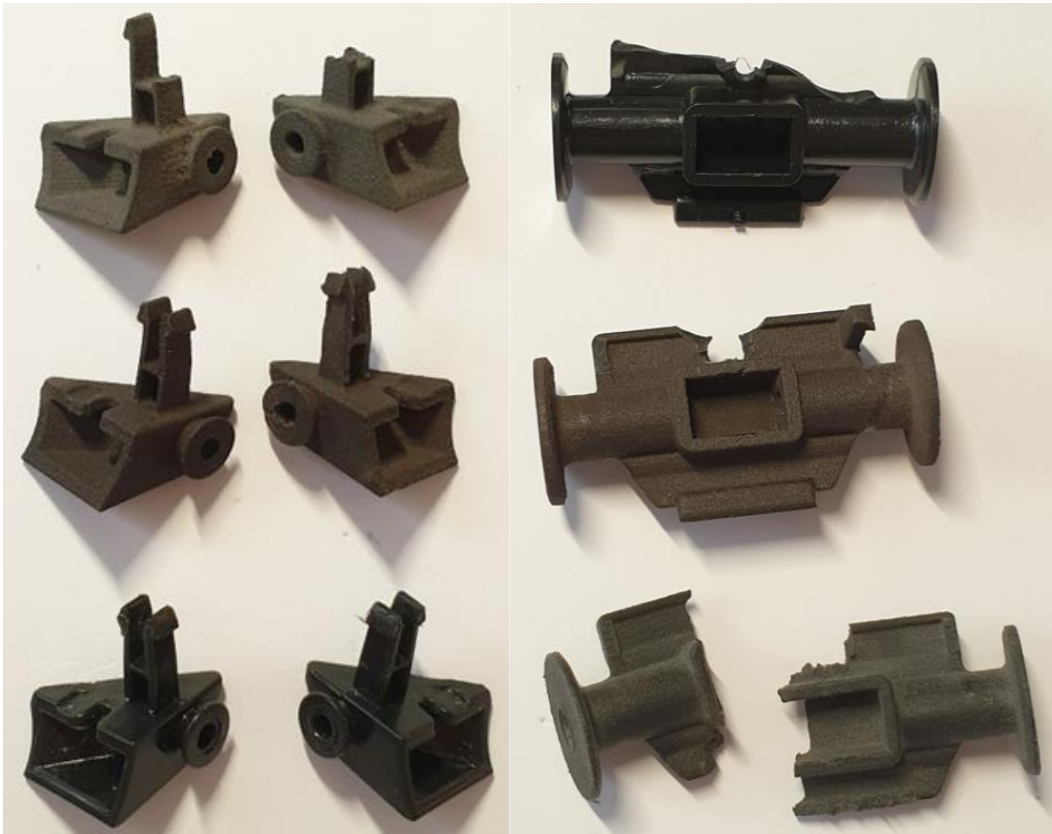
Figure 39: Outcomes from the conducted test. (Left) front wheel bearings, (Right) rear wheel housing. The GF 12 front bearing's exhibit a failure where two thin-walled cantilevered pillars are located, above a thicker-walled hollow structure. The rear housing PA 12 and original components present similar results, where the screw hole and the side snap fits present a brittle failure. In the case of GF 12, the structure was not strong enough, leading to complete structural failure.
