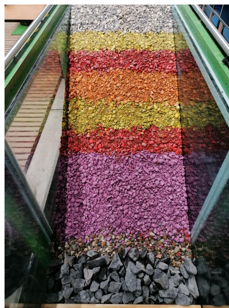
Figure 4.2: Under-layer after sub-series TS1.1
