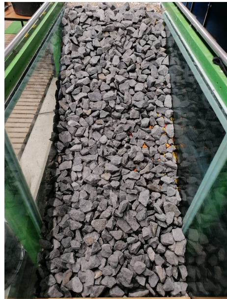
Figure 4.15: Armour layer after sub-series TS2.2
