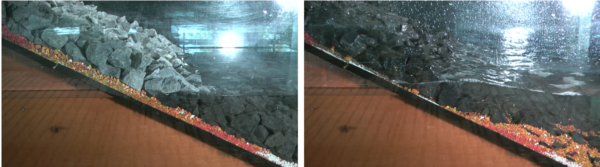
Figure 5.5: Side view of the filter structure. Left: Before test 3.2.1; Right: After test 3.2.3
