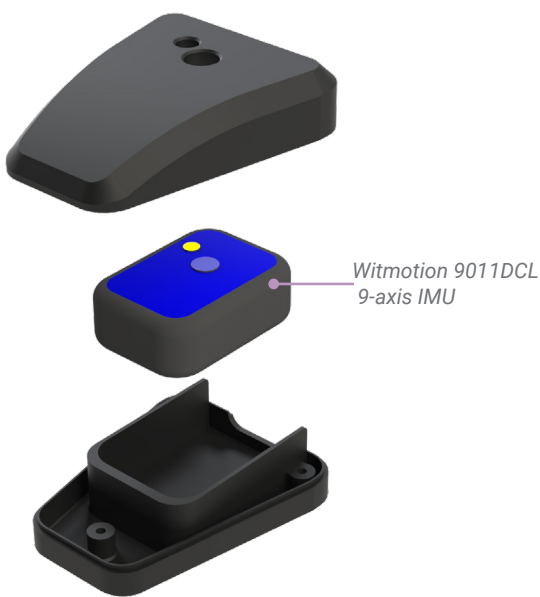
Figure 34: IMU case's assembly
