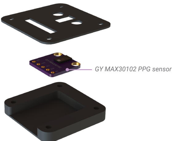
Figure 33: PPG holder assembly placed in the wriststrap
