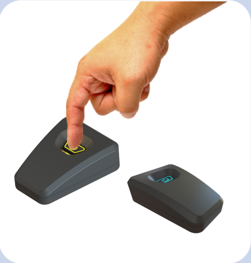
Step 2: Pressing the buttons on the modules to couple the sensors to your phone
