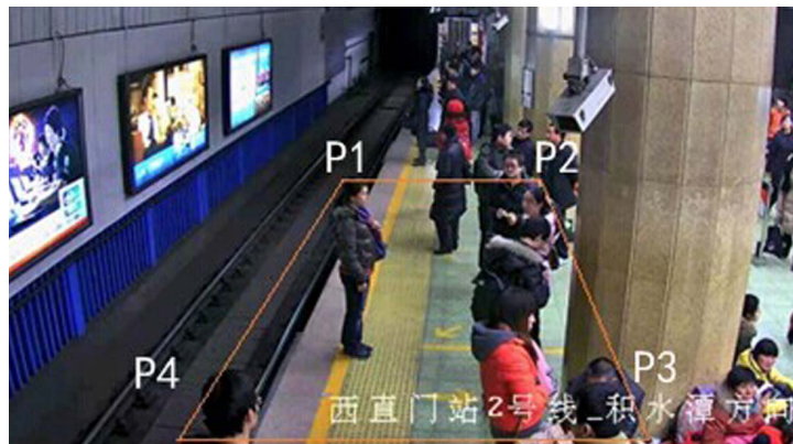
Fig. 1. Area of video detection, rectangle area enclosed by the four points P1, P2, P3 and P4.
