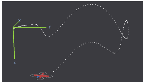
Figure 10.19: Simulation with drone path (white dots) determined by manual control inputs
