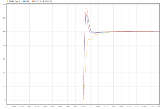
Figure 12: Step response of PID, PI^2D , PI(CI)D and PI^2D\_CgLP
