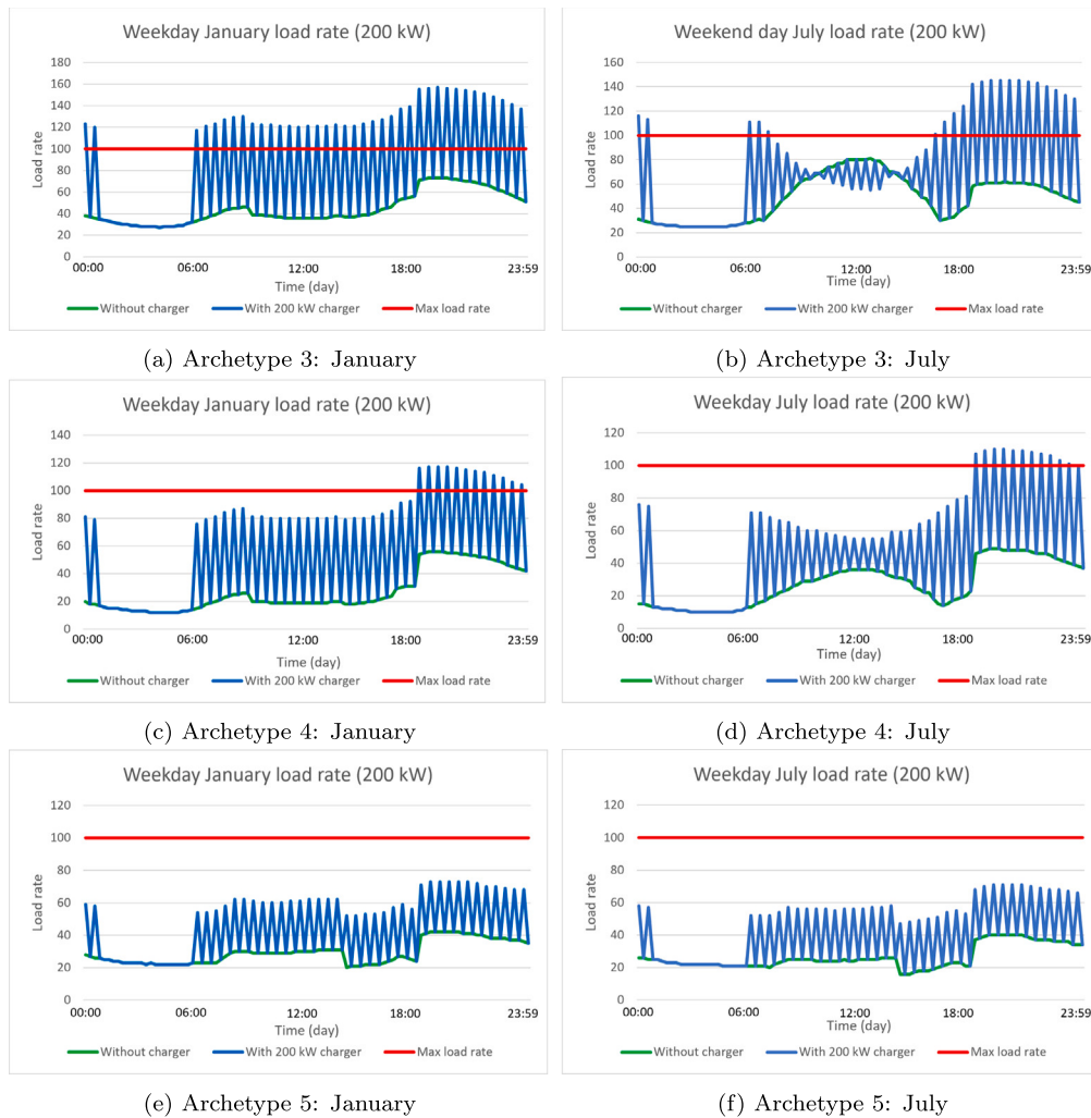
Fig. 11. The impact of a 200 kW charger on the grid of archetypes 3, 4 and 5: post-war terraced houses, post-war tenements, and corporation residences.
