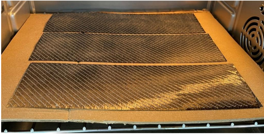
Figure 3.9: NCF plies in oven at the end of the 3-minute melting process (epoxy binder is molten and transparent)
