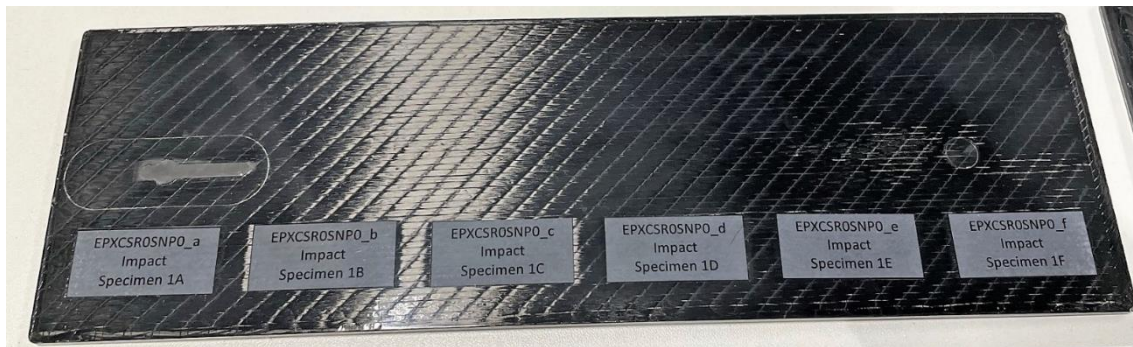
Figure 5.4: Impact specimens after the RTM process - dry spots are visible at the right side of the part
