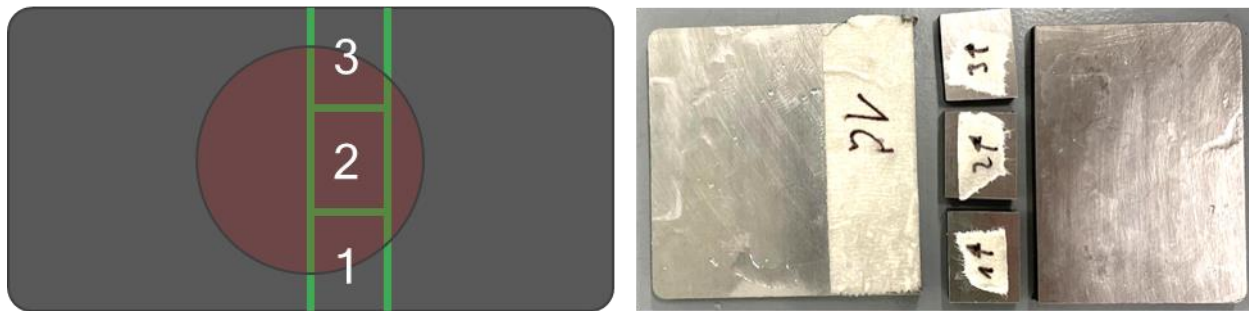
Figure 4.10: Sample cutting for microscopy (red highlights impact zone)
