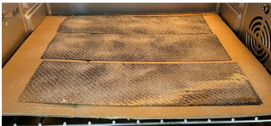
Figure 3.8: NCF plies in oven at the beginning of the 3-minute melting process (epoxy binder is still solid and whitish)
