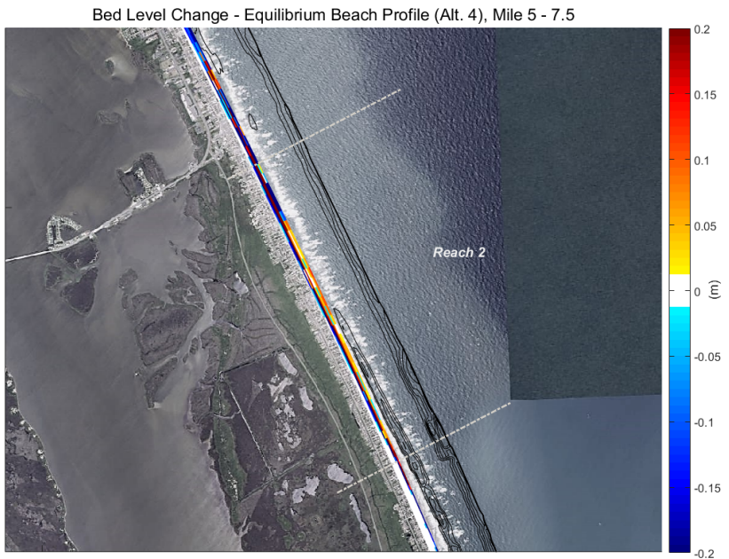
Figure D.6: Shoreface nourishment locations of alternatives 3 and 4 in mile 5 - 7.5 and its effect on the shoreline morphology
