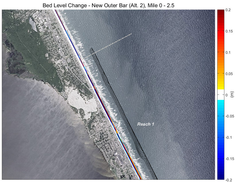
Figure D.1: Shoreface nourishment locations of alternatives 1 and 2 in mile 0 - 2.5 and its effect on the shoreline morphology
