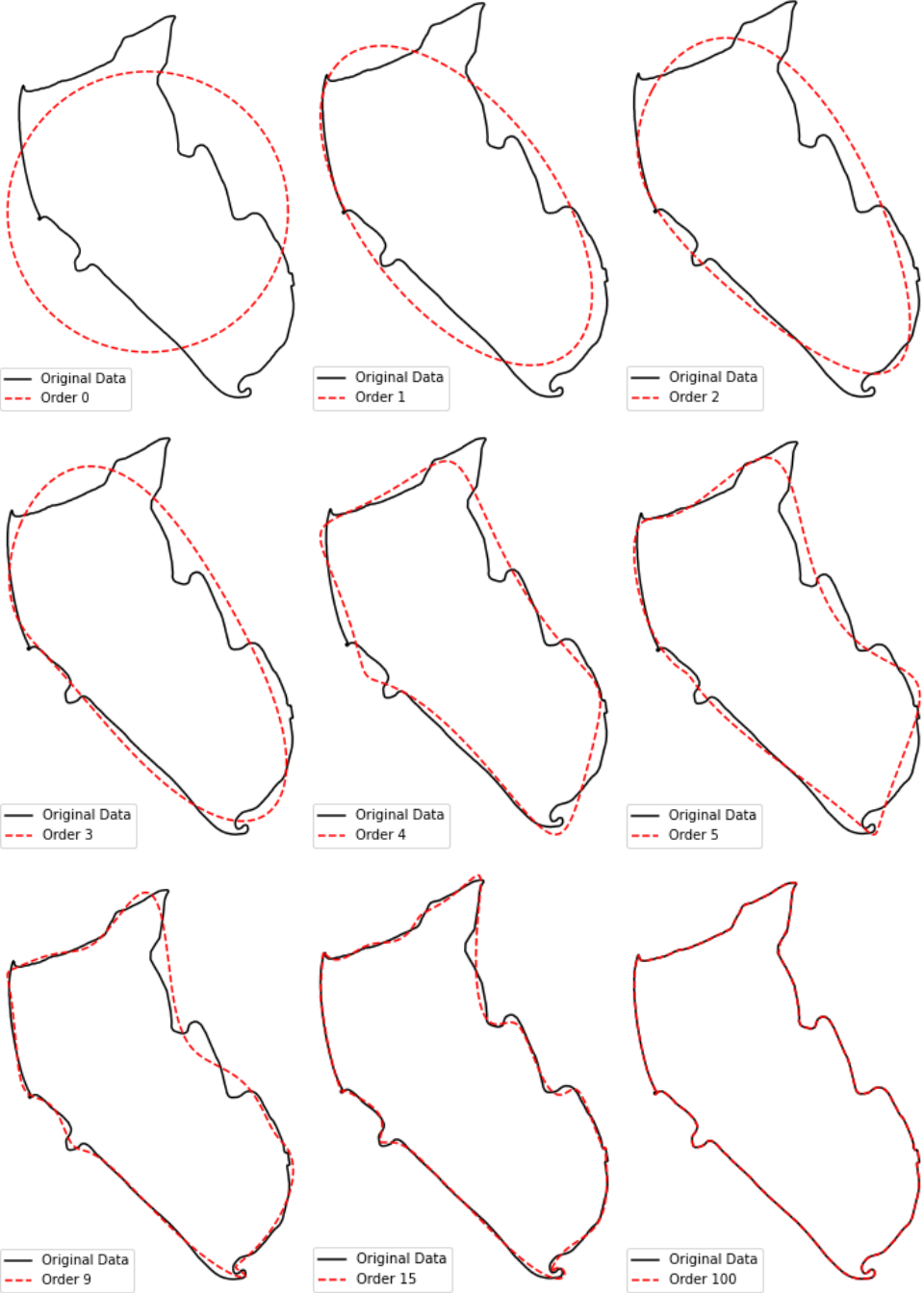
Figure 3.7.: Fourier transformation on the borders of the Marker Wadden. The black line indicates the original shape of the Marker Wadden. The dotted red line indicates the shape that is used in each Delft3D-Flow Nest model.
