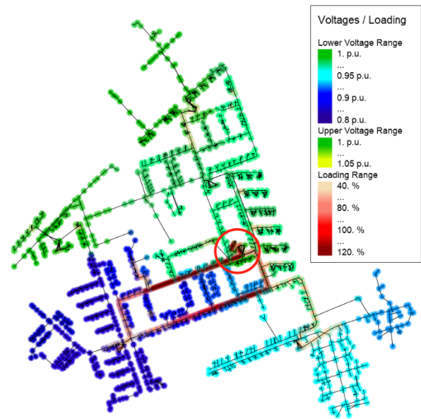
Fig. 1: Heat map showing the overloaded and under-voltage region in the suburban grid with 80% EV penetration.
