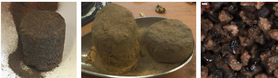
Figure 4.5: Cores from thermal treatments (upto 1050 °C) of two samples of Rock A (left and centre). Both tests resulted in a friable end product which could not be successfully cored over lengths in excess of roughly 3 cm. Magnified images of the thermally treated product (right) showing charring of organic matter (in black) over quartz grains. White bar on the top left corner of the image scales to 100 μm. The amount of clay in both the samples was not sufficient in order to maintain structural integrity of the sample upon sintering.
