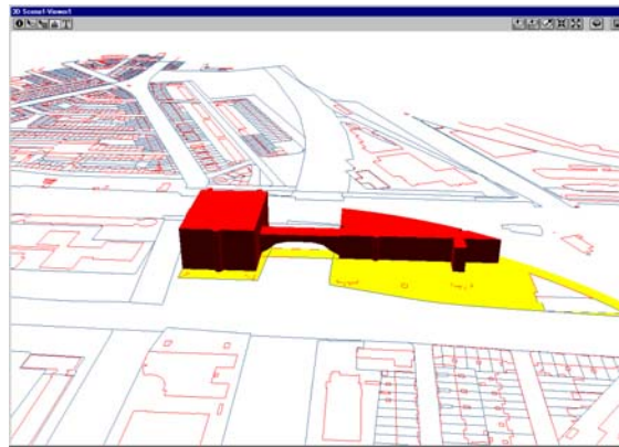
Figure 6: ArcView 3D Analyst representing the building, parcel boundaries and outlines of buildings. The coloured parcels are the result of the query: which parcels intersect with the projection of the building?
