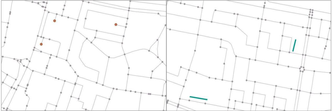
**Figure 4.3.** Topological errors: dead-ends (left), and isolated edges (right).
