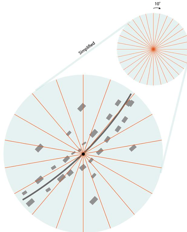
**Figure 4.11.** Rays casted from one sampling point
