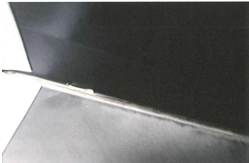
Figure 6.36: Enclosed release film in the corner section
