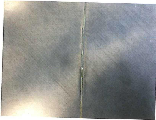
Figure 6.4: Filler indentations on the back of the skin of the panel along the filler location
