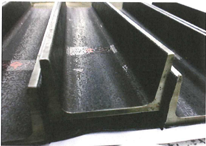
Figure 6.61: Hanging core on one side of the core with a height of 15 mm
