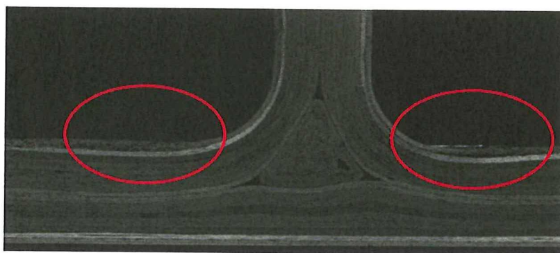
Figure 6.147: Resin rich areas in the corner sections of stringer 1
