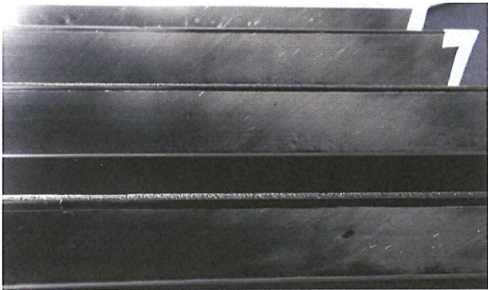
Figure 6.168: Slipped stringer plies in the stringers, with stringer 3 in the front
