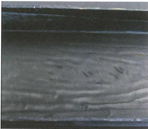
Figure 6.80: In-plane, undulations and the dry spots in the web of the stringer at core 3 where the hanging core was present
