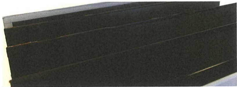
Figure 6.178: Slipped stringer plies with stringer 3 in the front
