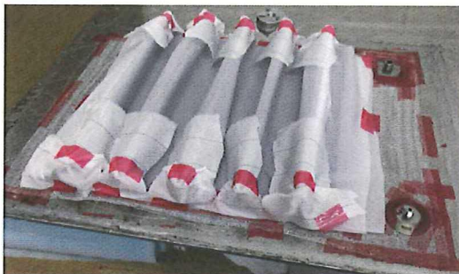
Figure 5.8: Application of airweave breather
