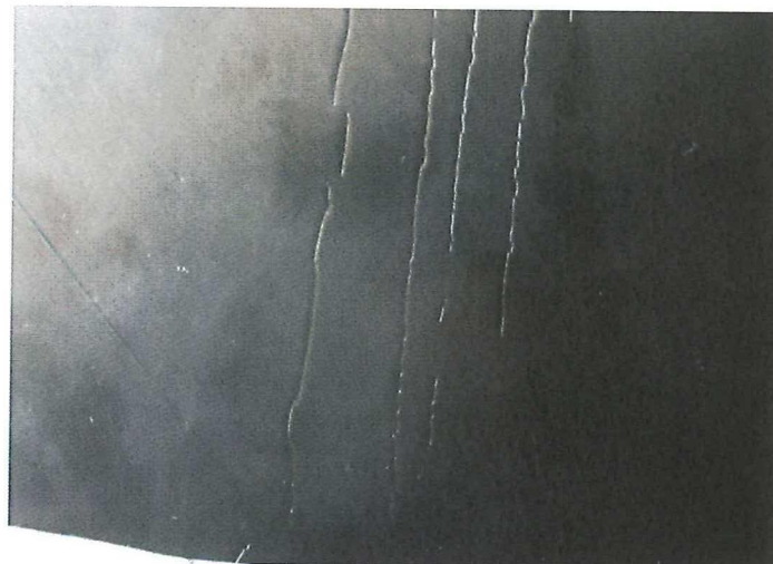
Figure 6.66: Out-of-plane waviness on the outer skin on the outer mould line
