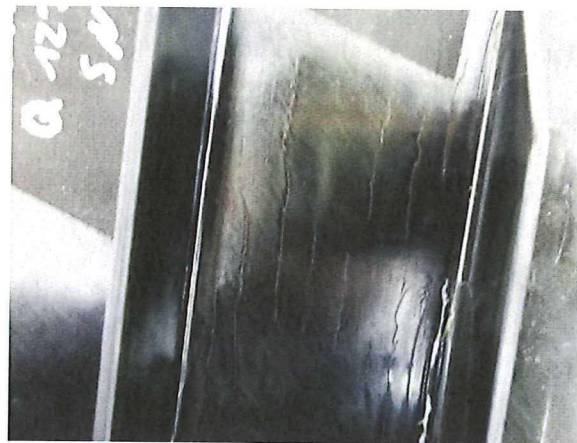
Figure 4.15: Out-of-plane waviness (undulations) on the outer surface
