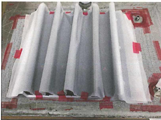
Figure 5.6: Application of release film over the cores
