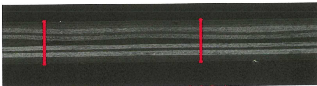
Figure 6.119: Out-of-plane undulations caused by the expansion of the layers in x-direction
