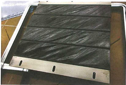
Figure 6.58: Waviness of the uncured stringer laminate on the outside of the stringer pack before turning
