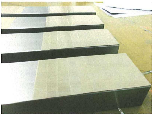
Figure 6.101: Inverted ramp on the tooling
