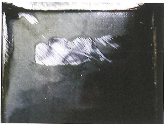
Figure 6.110: Dry spots at location 1 in core 4
