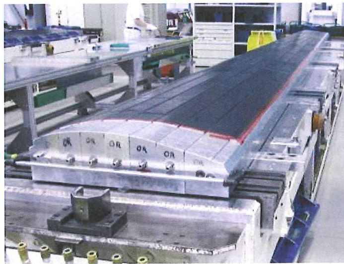
Figure 3.1: Compaction of the stiffener halves
