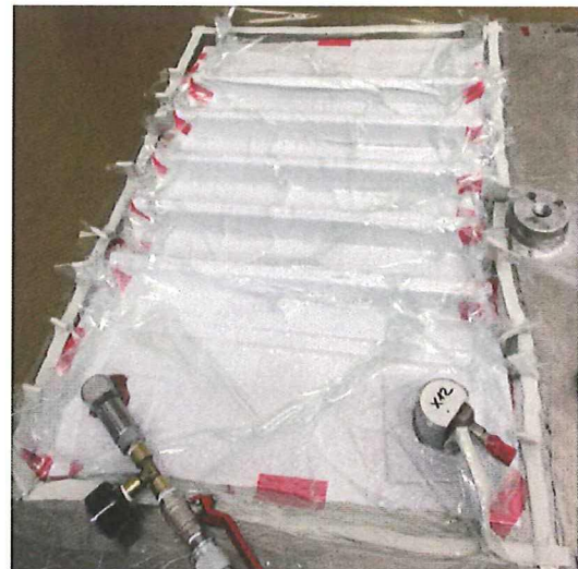
Figure 5.9: Application of the vacuum bag
