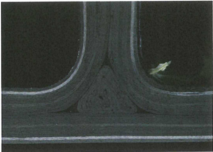
Figure 6.160: Resin rich areas in the corner sections as well as enclosed release film on the right side of the corner section in stringer 3
