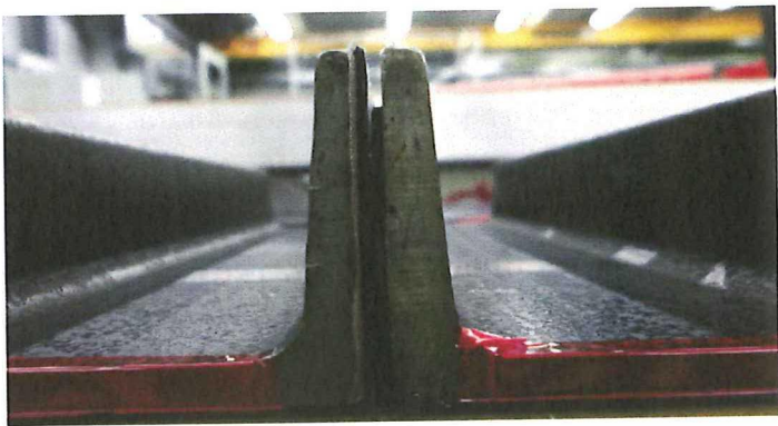
Figure 6.19: 8 mm shorter stringer laminate for core 3
