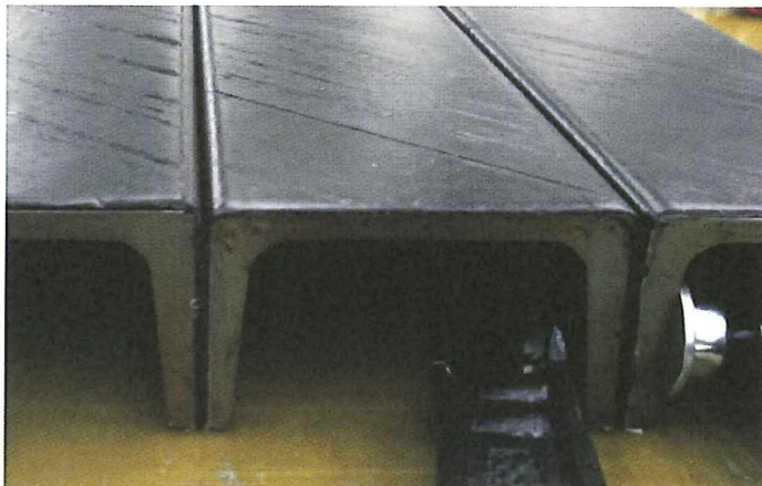
Figure 6.18: Good fit of the laminate around the corner sections of the core
