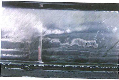
Figure 4.10: In-plane fibre waviness (undulations) on the surface
