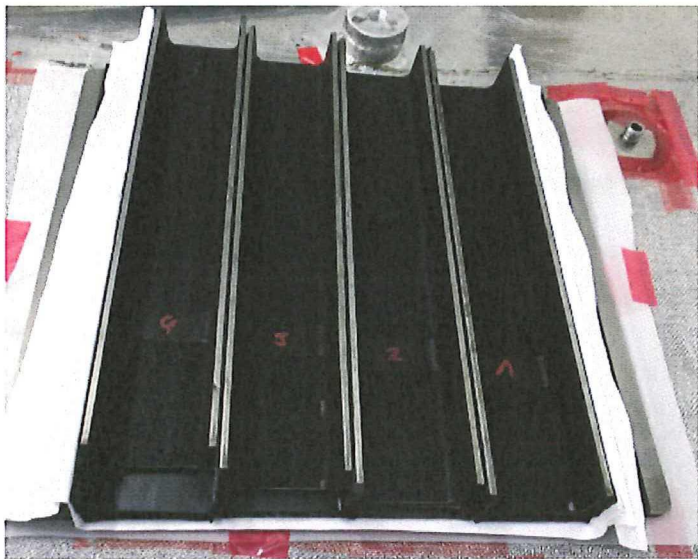
Figure 6.106: Shifting of the cores in the test part
