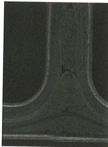
Figure 6.136: Vertical filler movement in stringer 2
