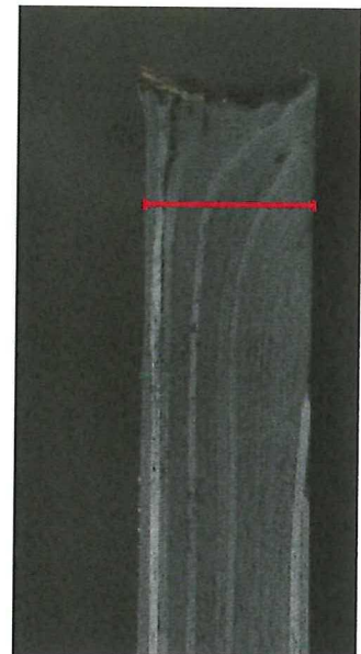
Figure 6.71: Slipped stringer plies of 6 mm in stringer 2 with the hanging core
