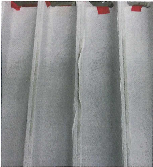
Figure 6.177: Brown stains in the airweave on top of the stringers after curing
