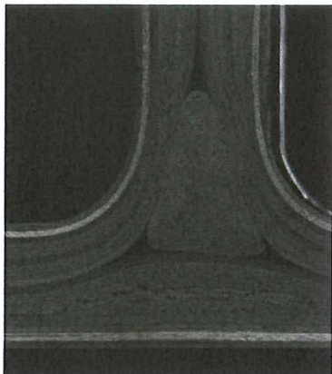
Figure 6.193: 150% filler material in the intersection of stringer 2
