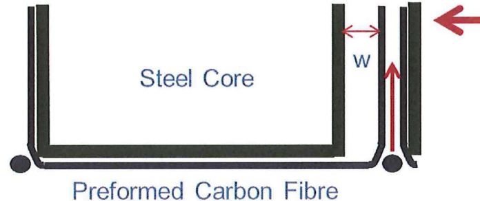
Figure 6.89: Graphical overview of the process alteration for when the steel autoclave cores are less wide than the preform cores
