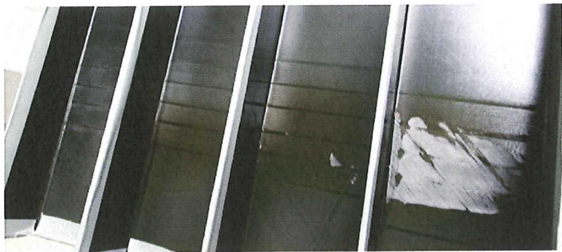
Figure 6.113: Increasing severity of brown areas for an increasing shifting distance
