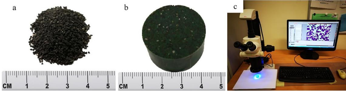
Fig. 5. Sand particles (a) and sample for image acquisition (b) under optimal microscope (c).
