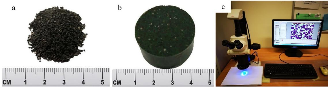
Fig. 5. Sand particles (a) and sample for image acquisition (b) under optimal microscope (c).
