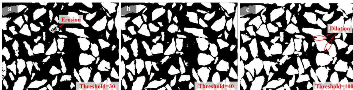
Fig. 10. Binary images after thresholding at (a) 30, (b) 40 and (c) 100.
