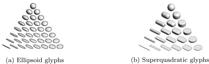
Fig. 2 Barycentric space of diffusion tensor shapes
