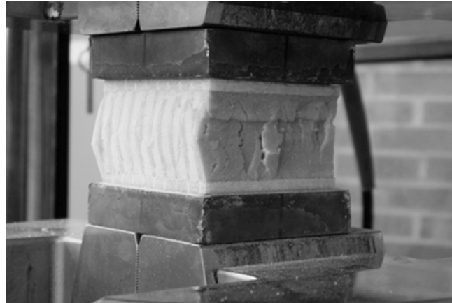
Figure 17: 3-D sandwich panel during compression test (source: Material characteristics of 3-D FRP sandwich panels )
