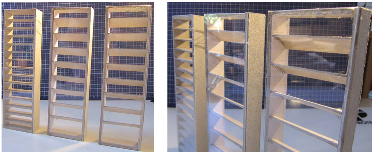
Figure 14: Practical models, testing the angel and shape of the sun shading profiles
