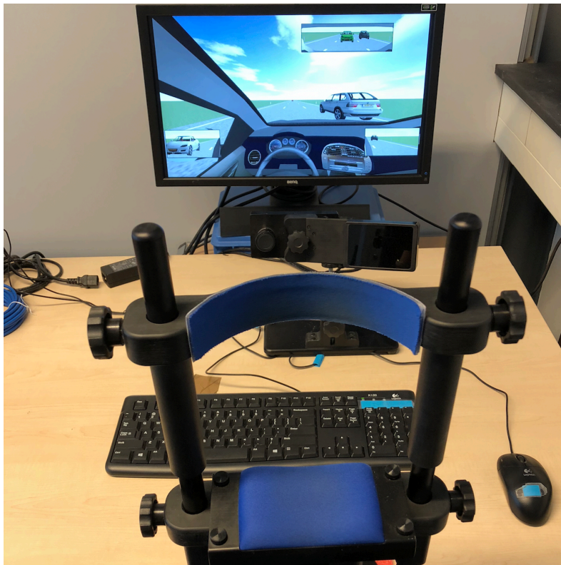
Figure 2. Experimental setup. In this picture is shown the head mount, Eyelink 1000 plus, the screen and input devices
