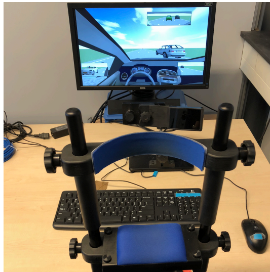
Figure 1. Picture of the experimental setup, in this picture is shown: The chin/head support, the keyboard, the eye-tracker and the computer screen.
