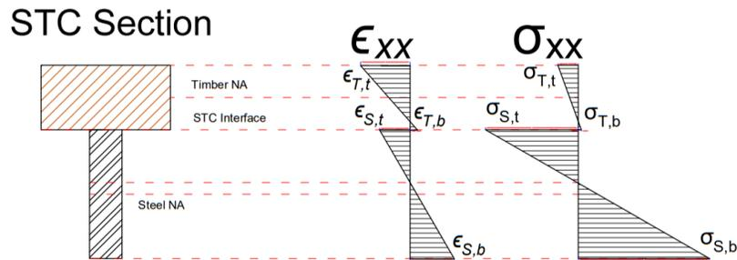
**Figure D.1: Normal Strains and Stresses for Elastic Analysis of STC.**
