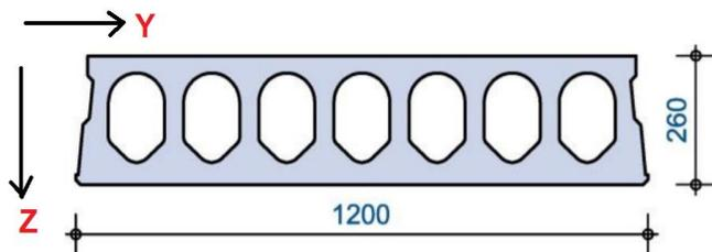
Figure 5.10: HCS260 Cross Section, adapted from [98].
