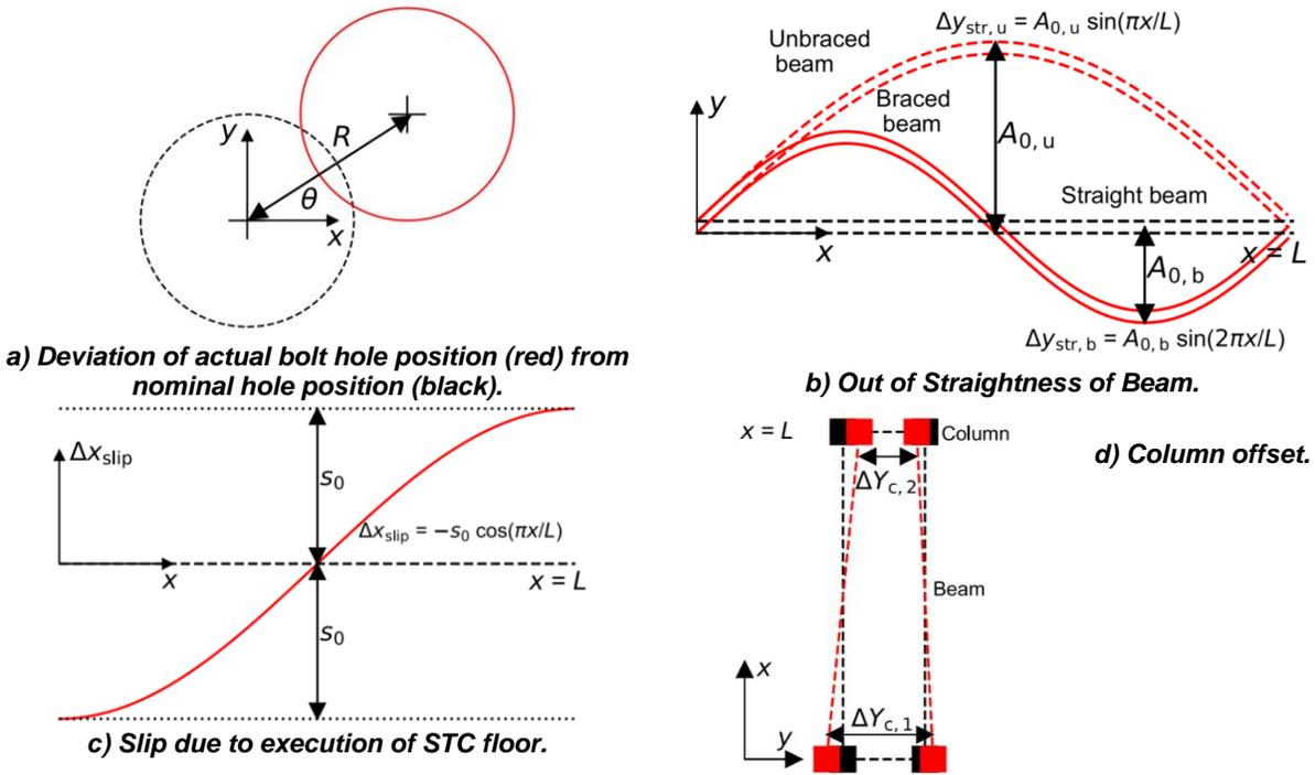
Figure D.3: Geometrical deviations in prefabricated floor systems, from [34].
