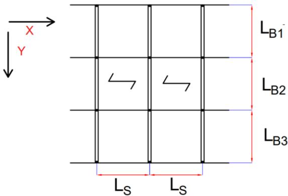
**Figure D.6: Structural scheme for Cocoon/Combination Office with HCS floor system.**
