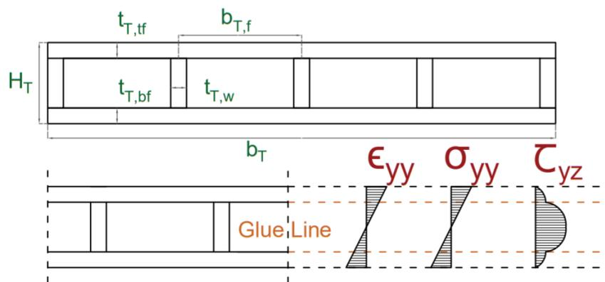
**Figure 6.1: Cross Section of LFE.**
