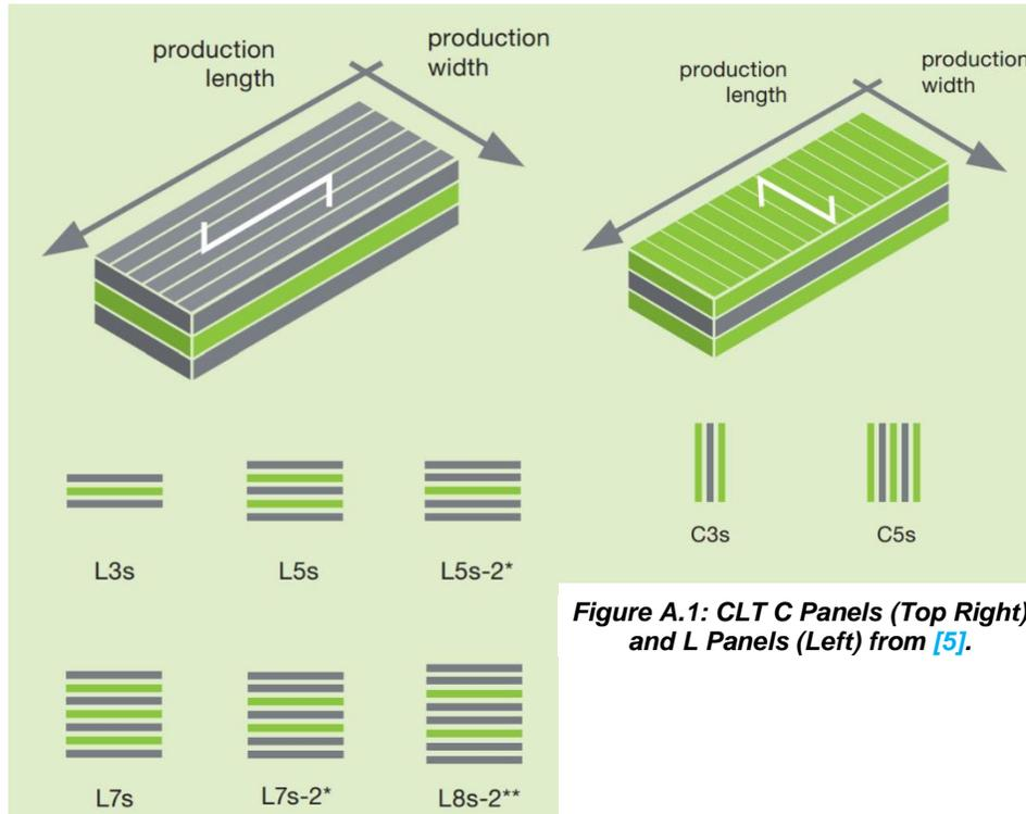
Figure A.1: CLT C Panels (Top Right) and L Panels (Left) from [5].
