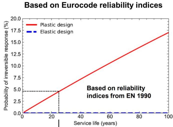
**Figure 2.4: Probability of Damage for Plastic and Elastic design of steel structures, adapted from [72].**
