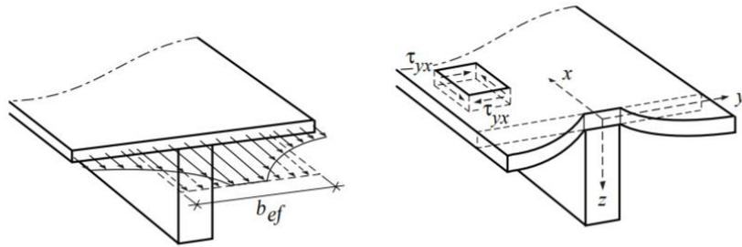
Figure 6.2: Stress Distribution in the Flange [3].
