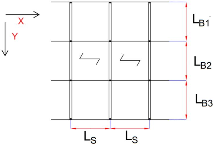
Timber Slabs (LFE) spanning in x-direction, supported by I-Beams (HEA)
