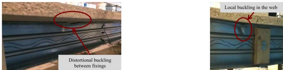
**Figure 3.10 Failure Modes in STC beams with *CLT* and cold formed C-sections, from [17]. (Left) Distortional Buckling. (Right) Web local buckling.**
