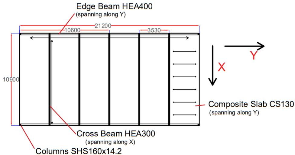
**Figure 5.12: Floor Plan of DA3\_CS.**
