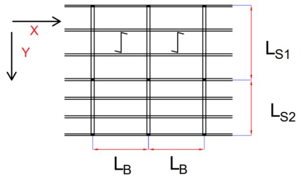
Figure D.9: Structural Scheme for Cell Office with Composite Slab floor system.
