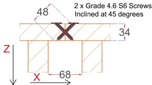
**Figure 5.7: Slab - Slab connections for Timber.**
