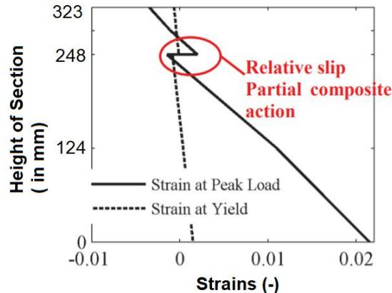
**Figure 6.4: Strain Distribution of STC Section from Hassanieh's Experiments, adapted from [24]. The results shown here are for Steel - LVL specimens with Coach Screws as shear connectors (Specimen #4).**
