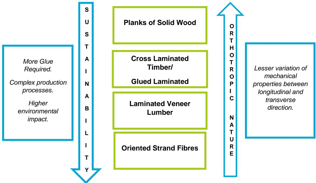
Figure 3.1: Comparison of Different Engineered Timber Products
