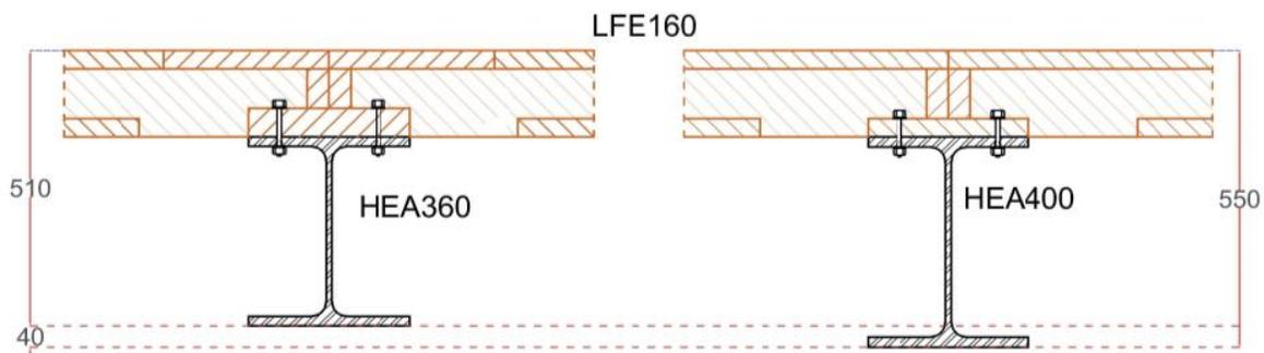
Figure 5.14: Comparison of *STC* with/without Composite Action.
