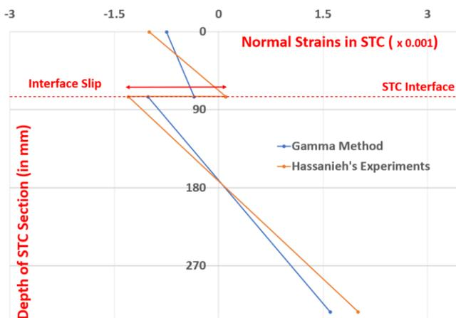
Figure 6.6: Distribution of Normal Strains over depth of STC. Comparison between Gamma Method and Experimental values.
