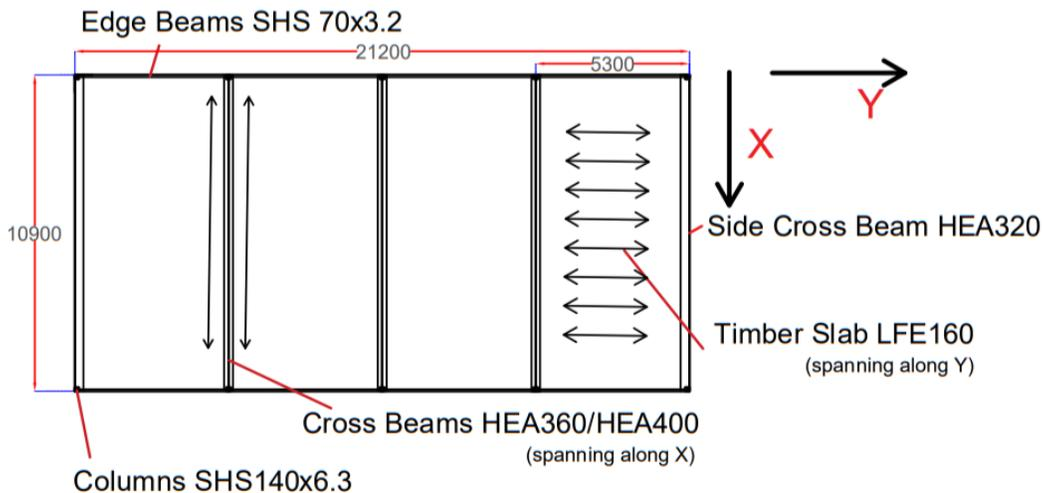
**Figure 5.5: Floor Plan of DA1\_STC.**
