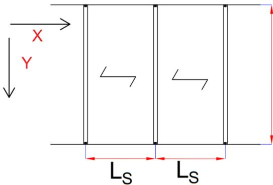
$L_B$  Timber Slabs (LFE) spanning in x-direction, supported by I-Beams (HEA).
