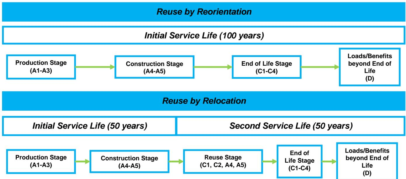
Figure 7.1: Modelling Reuse in LCA.
