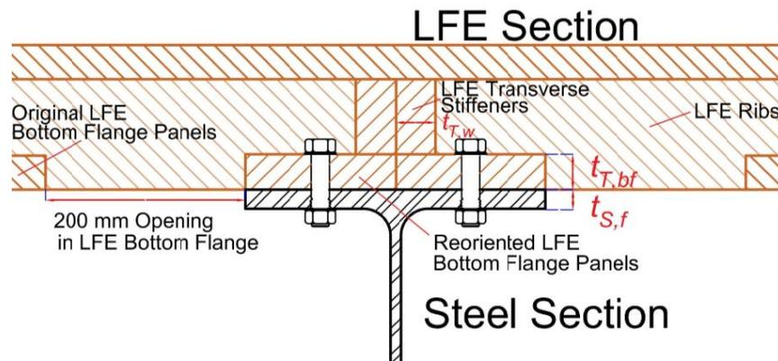
Figure 6.7: Steel Timber connection with Bolts.
