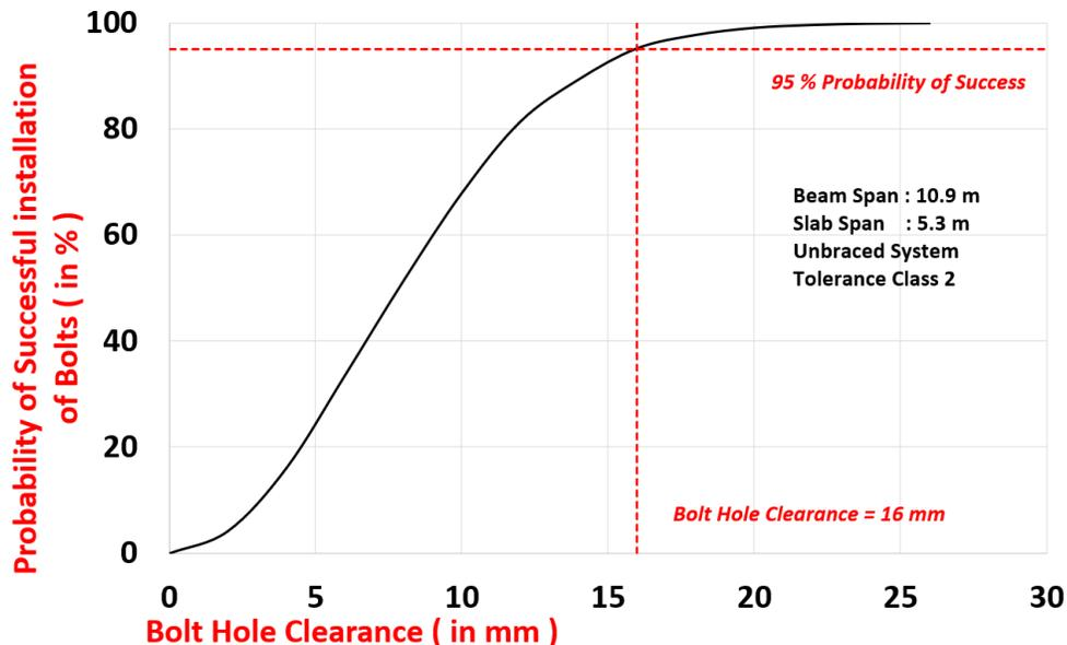
Figure 6.9: Probability of successful installation of bolts designed to be demountable.
