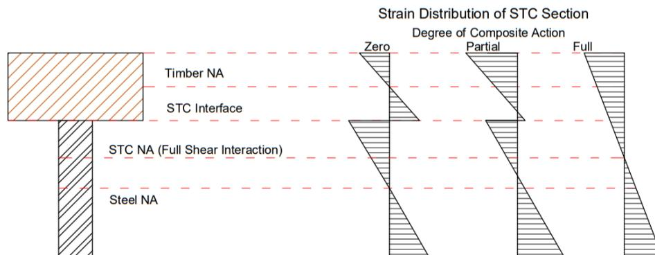
**Figure 6.3: Distribution of Normal Strains in STC Section for varying degrees of Composite Action. (Left) No Composite Action. (Middle) Partial Composite Action. (Right) Full Composite Action.**
