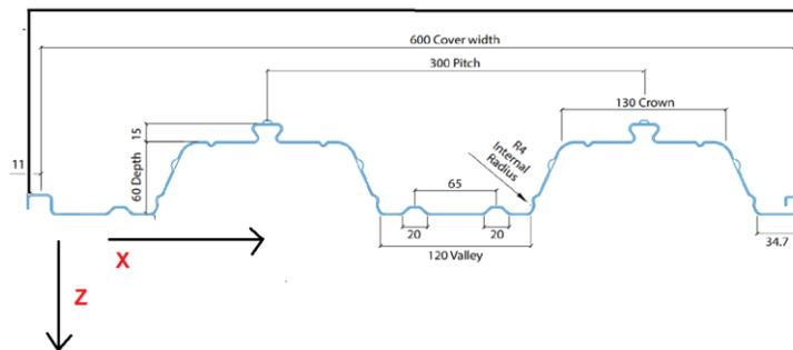
Figure 5.13: CS130 Cross Section, adapted from [99].
