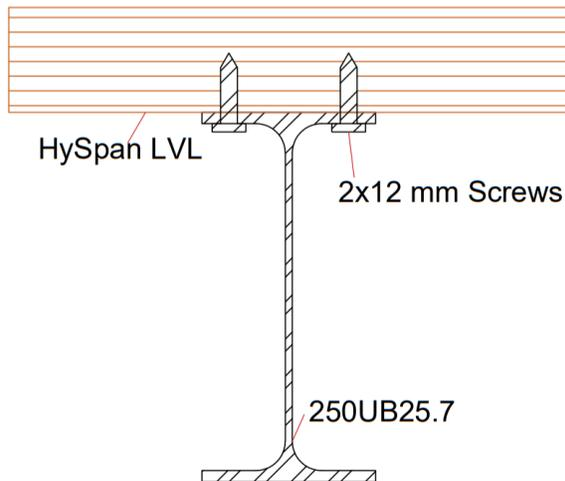
Figure 6.5: Steel - LVL composite from Hassanieh's experiments. Specimen #4, from [24].
