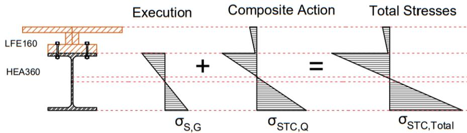
**Figure 6.12: Load mechanism of STC Section, showing the distribution of normal stresses.**
