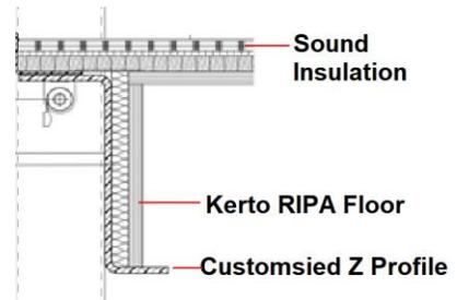
Figure 5.3: Customised Z Profile supporting Kerto RIPA floor elements.
