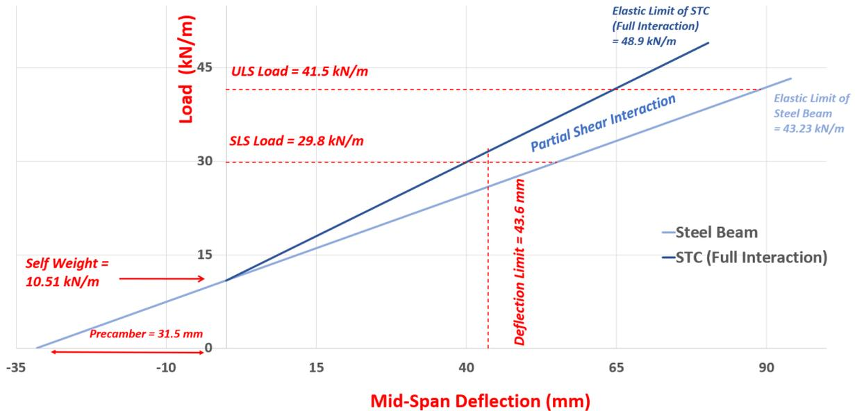
**Figure 6.11: Load - Deflection Curve of the STC Beam.**
