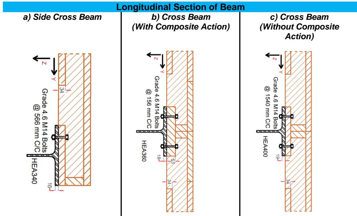
**Figure 5.8: Slab - Cross Beam Connections.**
