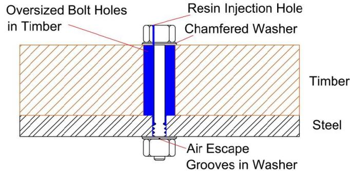
**Figure 8.2: Proposed Resin Injected Bolted Connection with Oversize Hole in Timber.**
