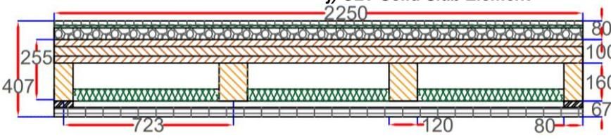
**k) CLT Open Rib Element**
