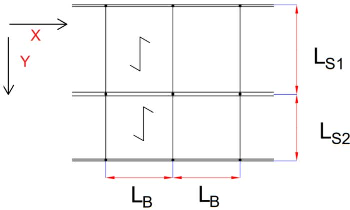
Timber Slabs (LFE) spanning in y-direction, from façade to façade, supported by I-Beams (HEA), with an intermediate support.
