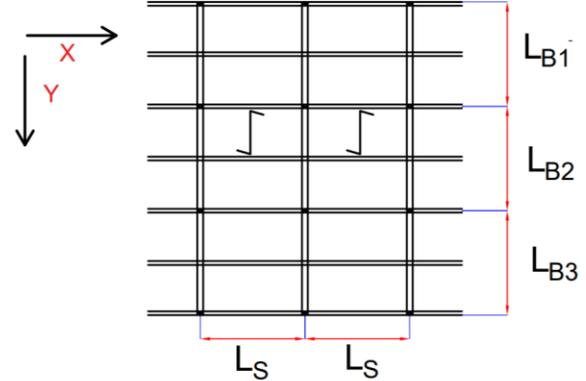
**Figure D.7: Structural Scheme for Cocoon/Combination Office with Composite Slab floor system.**
