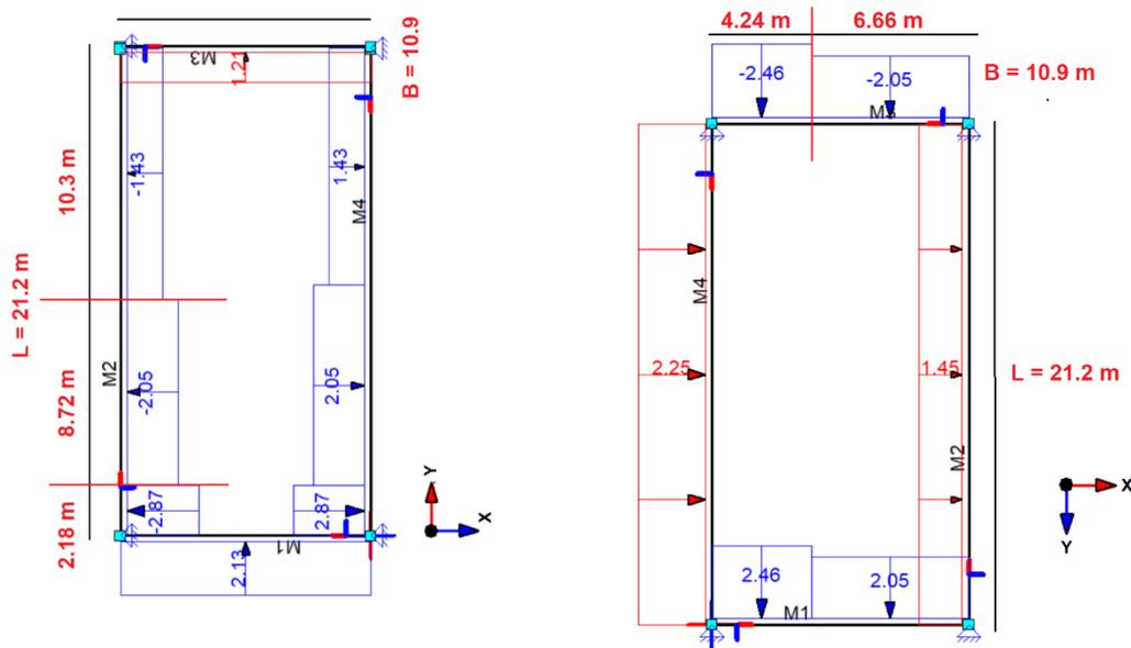
Figure 5.4: Wind Loads on Top Storey. (Right) Wind acting perpendicular to Long side. (Left) Wind acting perpendicular to Short side.
