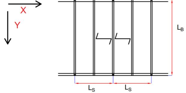
Figure D.11: Structural Scheme for Group Office with Composite Slab floor system.
