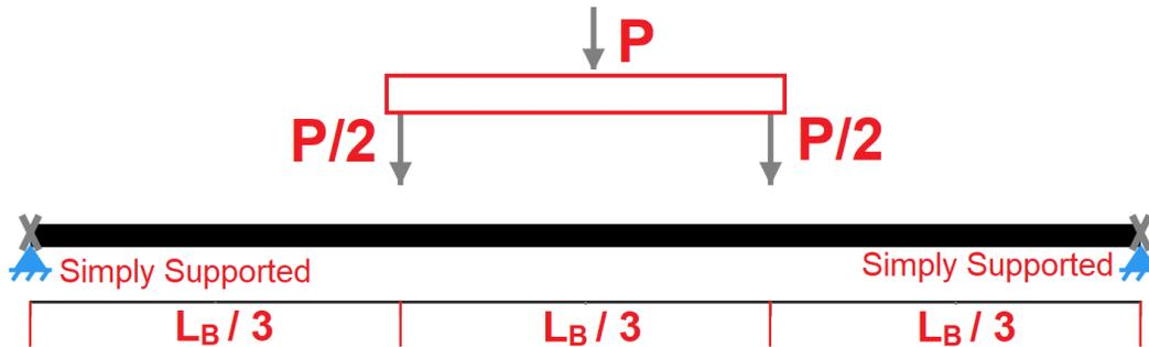
**Figure D.2: Structural Scheme of Hassanieh's Experiments. 4-Point Bending.**
