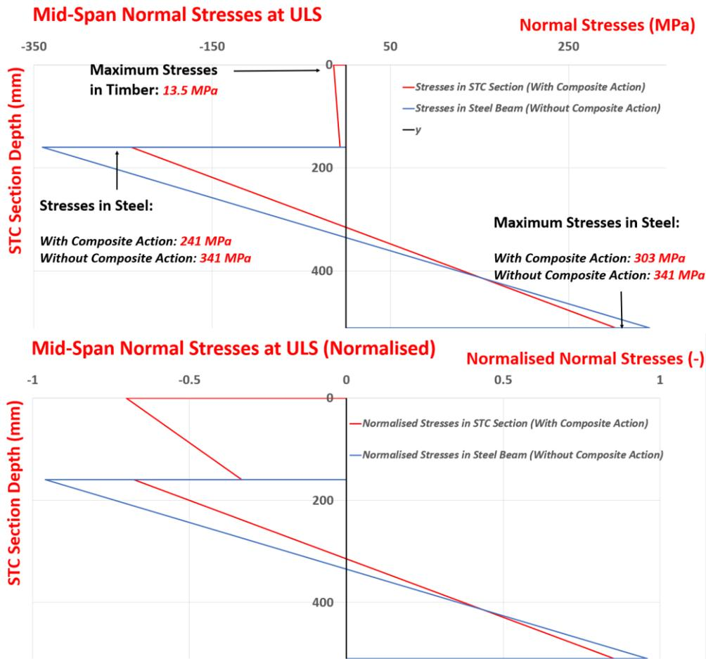
Figure 6.13: Stresses in the STC Section. (Top) Values in MPa. (Bottom) Values normalised to bending strengths of steel/timber.
