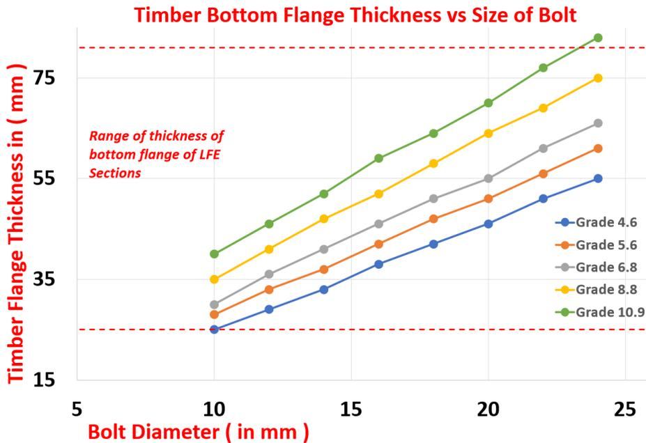
Figure 6.8: Thickness of timber bottom flange vs Bolt Diameter for different grades of Bolts.
