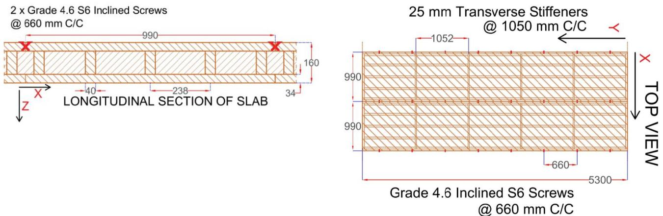
Figure 5.6: Dimensions of Timber Slab, LFE160.
