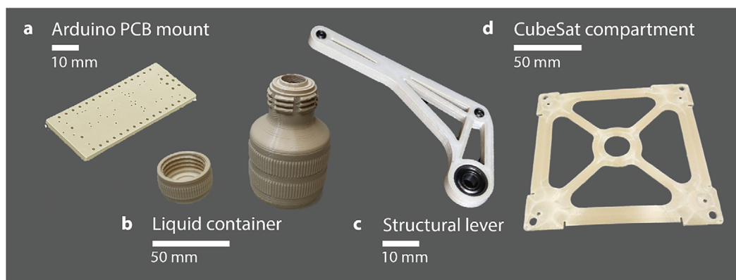
Figure 9. Possible use cases of 3D-printed LCP in space, with different scales of application manufactured with different 3D printers: A) an Arduino PCB mount, B) a screw-cap liquid container, C) a structural lever with bearings, and D) a compartment panel for a CubeSat.
