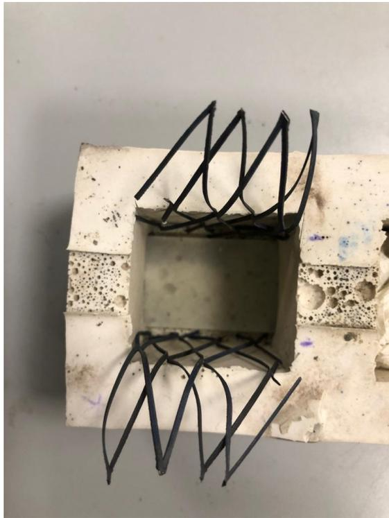
Figure 3: Mould setup for the setting time test
