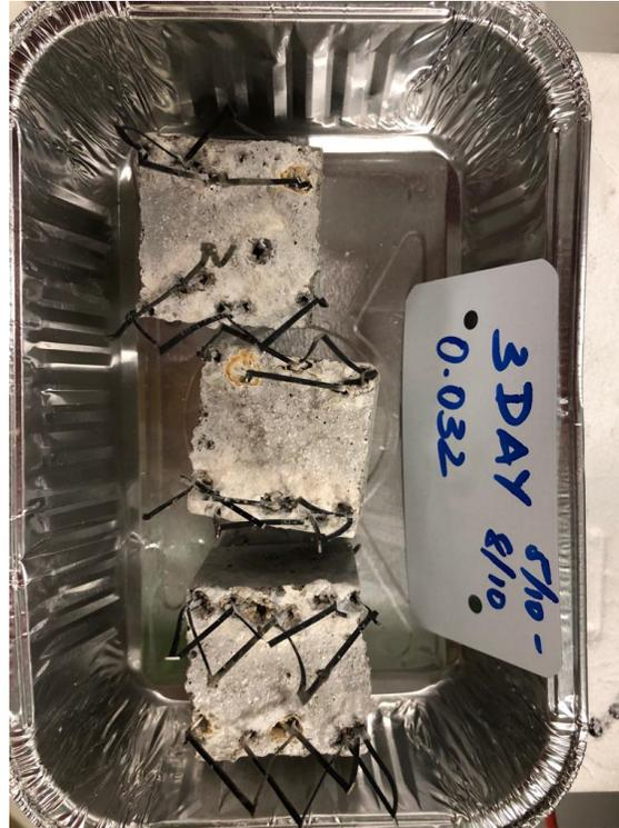
Figure 31: 20 A/m<sup>2</sup> samples prepared for a 3-day compressive strength test
