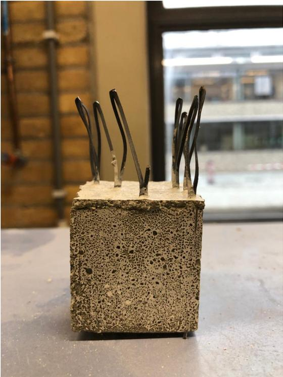
Figure 4: Cube specimen subjected to electric curing
