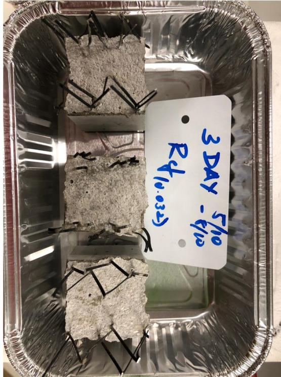
Figure 32: Control samples (without application of current) prepared for a 3-day compressive strength test
