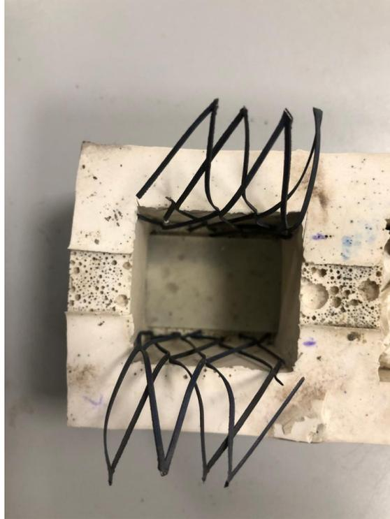
Figure 14: Box mould with electrodes
