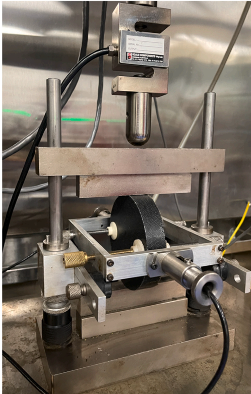
Fig. 8. Setup of indirect tensile stiffness modulus test.
