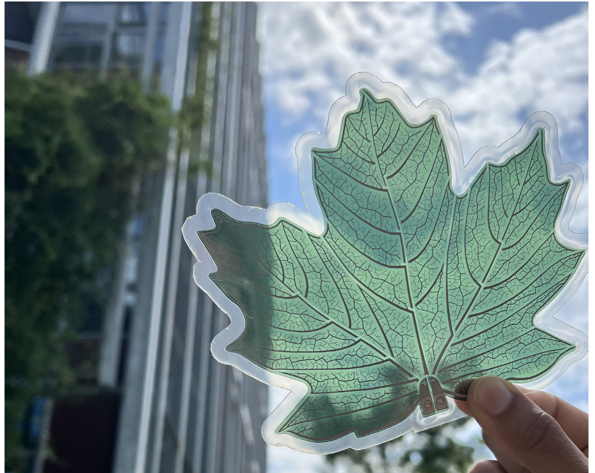
ORGANIC PHOTOVOLTAIC FILM IS SEMI-TRANSPARENT AND CAN BE MADE IN DIFFERENT SHAPES AND COLOURS
