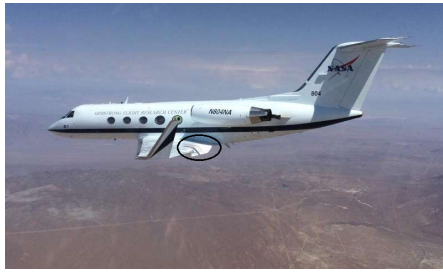
(a) NASA Armstrong's G-III during flight test for the Adaptive Compliant Trailing Edge (ACTE) project
