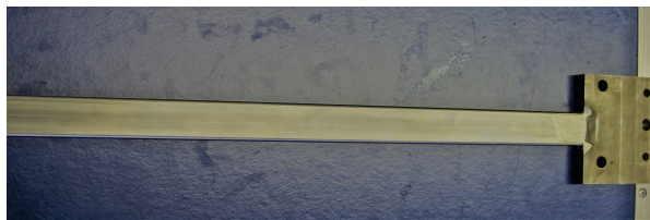
Figure 4.4: Interface rod to mount the wing in the test section
