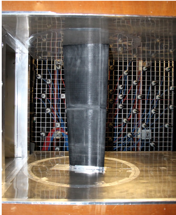
Figure 4.11: View of the wing(morphed) fitted between side-plates and in front of the microphone array
