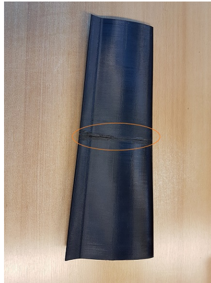
Figure 4.6: Morphed wing glued after 3D printing with glued surface highlighted
