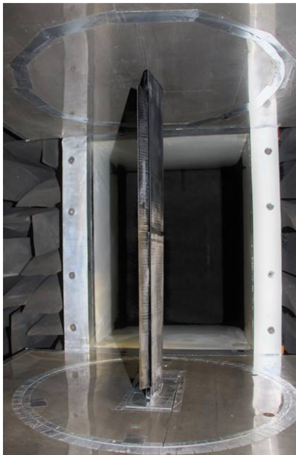
Figure 4.9: Wing profile mounted between two horizontal side-plates
