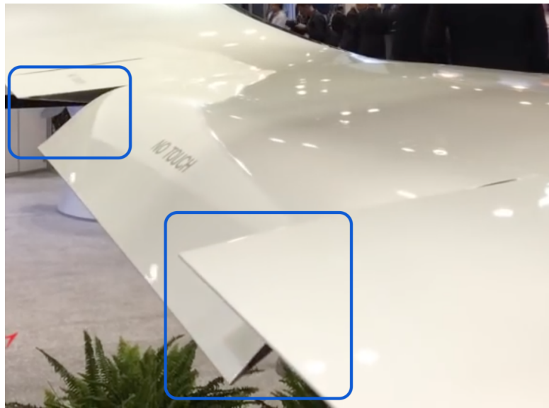
Figure 3.12: Flexsys morphing wing concept with side-edges highlighted
