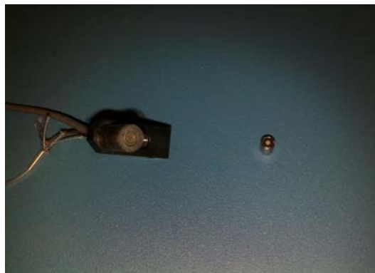
Figure 4.17: Endeveco 8507-C pressure transducer and Sonion 8010T microphone
