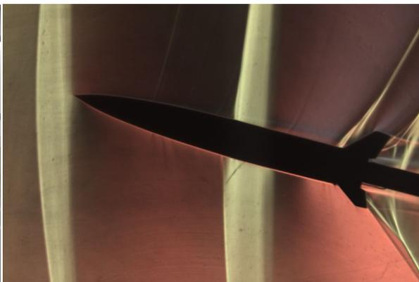
Figure 2.21: PRORA Unmanned Space Vehicle developed by Italian Aerospace Research Center (CIRA) [25]. Figure 2.22: Schlieren image of wind tunnel model of the PRORA-USV. [24]
