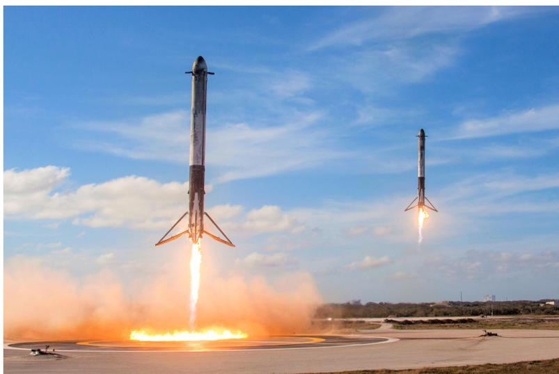
Figure 1.1: Side boosters of Falcon Heavy performing vertical landing at Kennedy Space Center [2].
