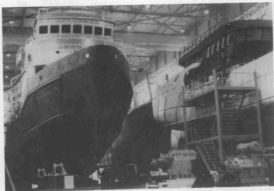
Photo 2. Construction with steel hull and aluminium superstructure
