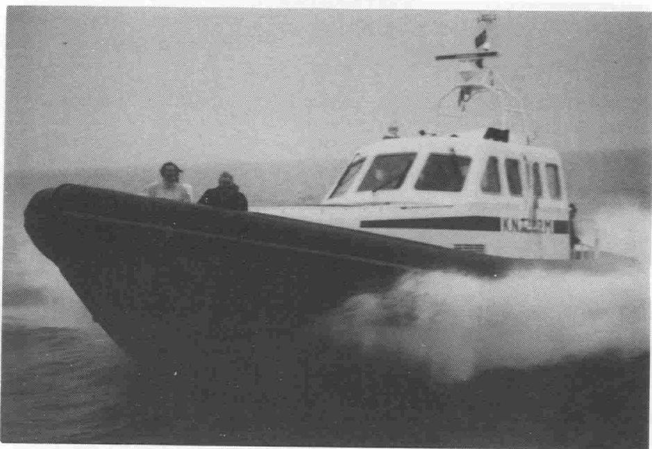
Photo 4. Lifeboat, completely constructed of aluminium
