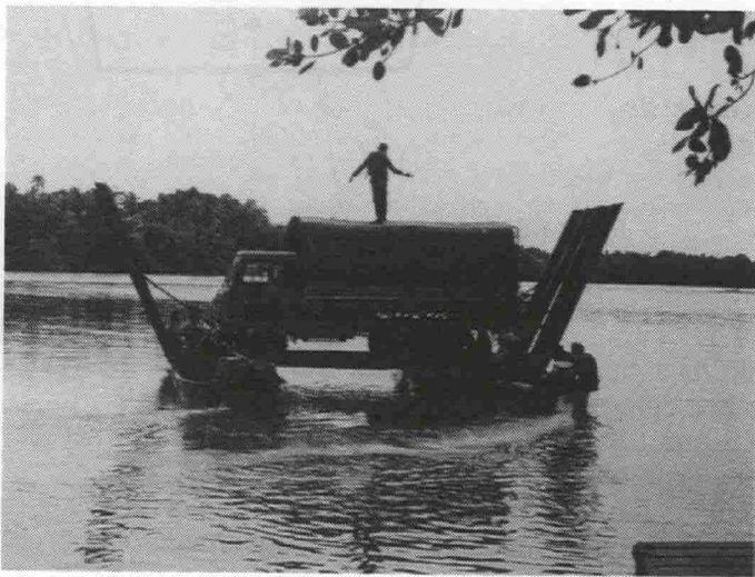
Figure 7 Four Damen assault craft in a catamaran configuration for an MLC.6 raft
