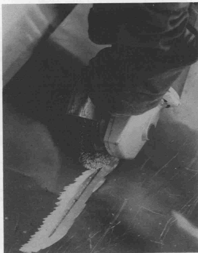
Photo 13. Removing the oxide layer by grinding
