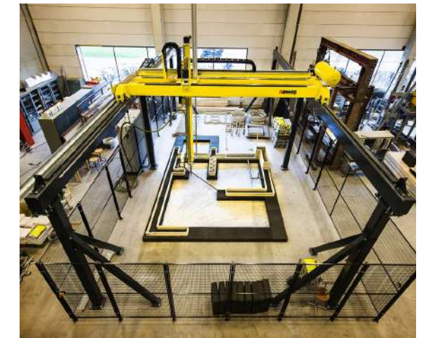
Figure 5.5: An example of a gantry system for large scale concrete printing, via TU Eindhoven
