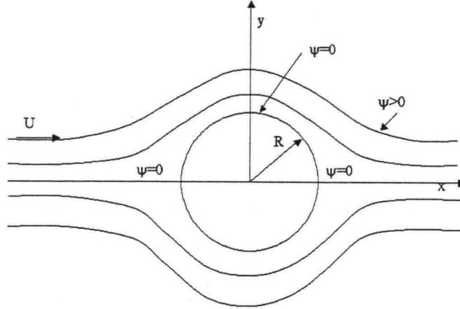
Figure 3.2: Streamlines of ideal flow around an impermeable circle
