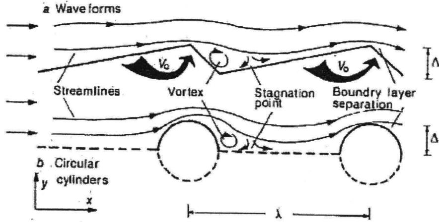
Figure 3.1: Analogies of flow conditions around objects in a flow field. a) Over-bed and in-bed flow for a sandwave bedform. b) Flow across cylinders. (Thibodeaux & Boyle, 1987)
