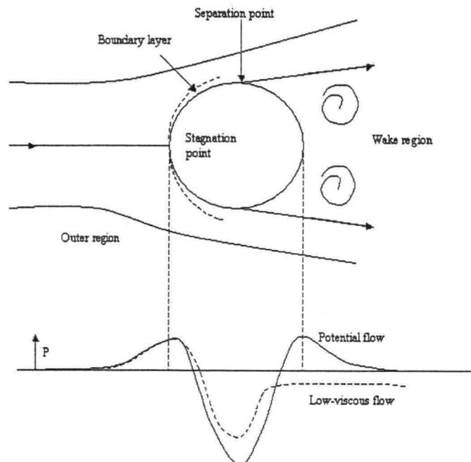
Figure 3.3: Low-viscous flow and pressure distribution around an impermeable circle.
