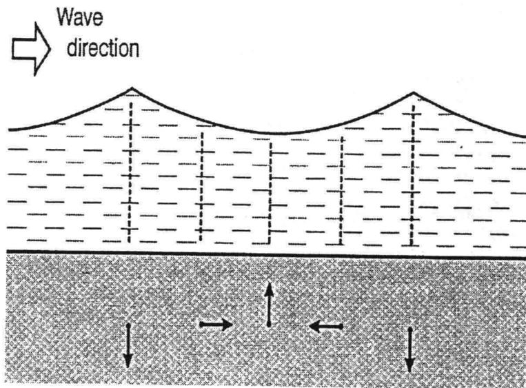
Figure 3.8: Pressure induced by waves over a flat bed
