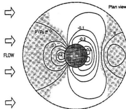
Figure 3.5: Pressure field around a hemisphere according to windtunnel measurements by Taniguchi & Sakamoto (1982) produced by Huettel & Webster (2001). Lines present isobars.
