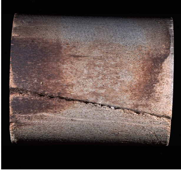
Figure 18: Side view from a core sample baked at 900 °C
