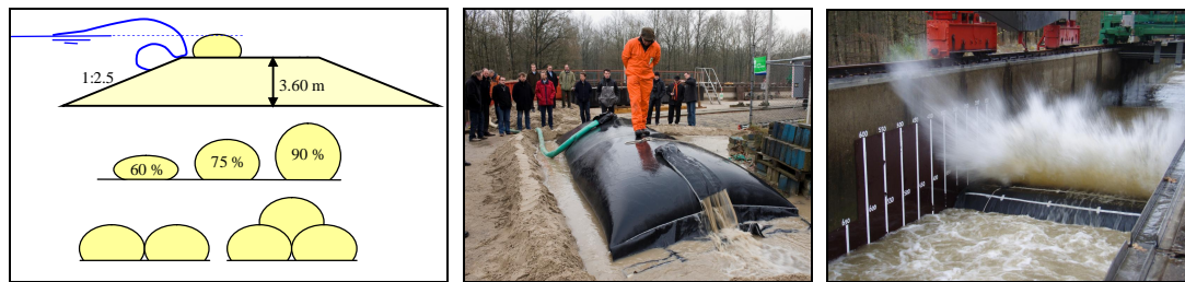
Figure 2. Schematized test set-up of geotextile tubes; filling of tubes (demonstration besides flume); test-run
